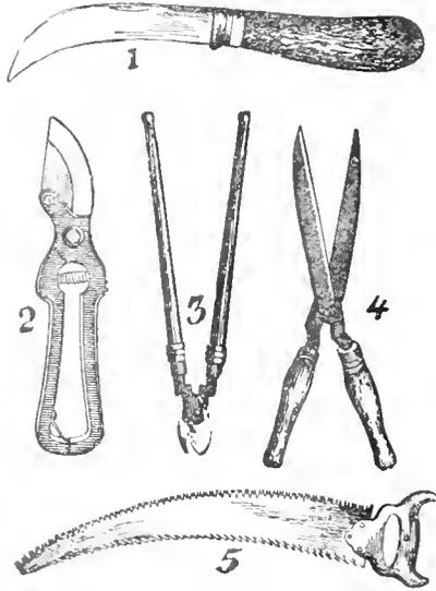
1. Hawkbill knife for small trees and larger branches. 2. Hand pruner shears for still larger branches. 3. Lopping shears for pruning hedges. 4. Shears for pruning hedges. 5. A very desirable form of pruning saw.
