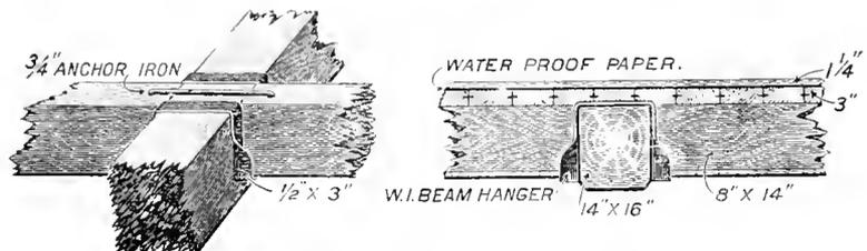
DETAILS OF FLOOR AND OF FLOOR BEAMS.
