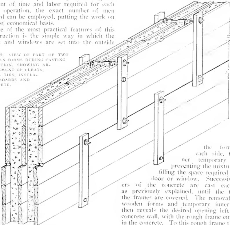
the forms on each side, the inner temporary frame preventing the mixture from filling the space required for the door or window. Successive layers of the concrete are cast each day, as previously explained, until the tops of the frames are covered. The removal of the wooden forms and temporary inner frame then reveals the desired opening left in the concrete wall, with the rough frame embedded in the concrete. To this rough frame the door
