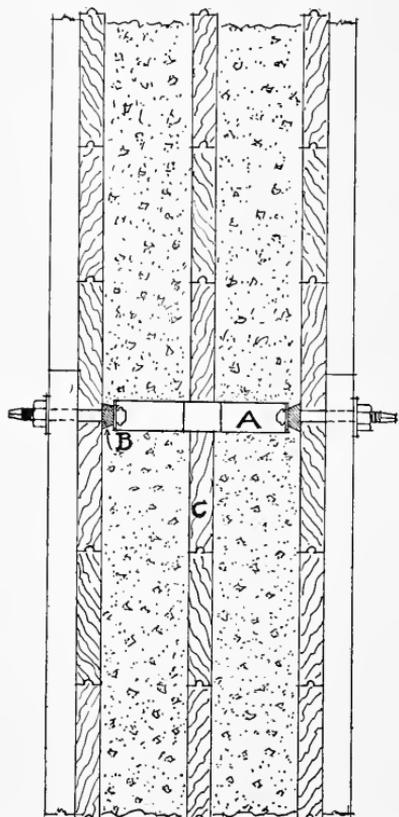
FIG. 2: VERTICAL SECTION THROUGH TWO OF THE WOODEN FORMS USED IN CONSTRUCTION OF BUNGALOWS NOS. 131 AND 132, SHOWING CENTRAL INSULATING BOARDS EMBEDDED IN CONCRETE AND HELD IN PLACE BY METAL REINFORCING TIE.
