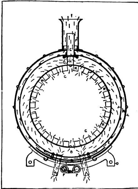
FIG. 165.—Cross-section of Sprague hot dry-air apparatus : A, A, air intakes ; a, circulating air space ; b, jacketed space for products of combustion ; G, treatment-chamber ; M, M, cork ribs ; N, N, perforations admitting heated air ; o, base holding apparatus ; P, P, gas-burners.
