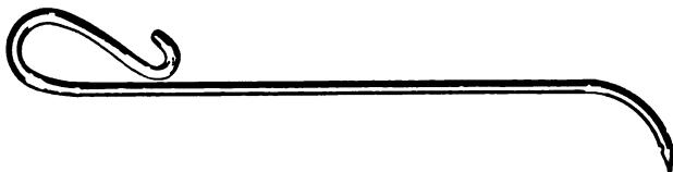
FIG. 158.—Needle specially designed to carry a thick wire. The eye is drilled obliquely, and should receive only a little loop on the end of the wire ; this loop should be made previously.
