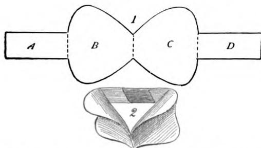
FIG. 152.—1. Diagram showing outline of Van Arsdale's splint. The end band to be folded on the dotted lines; each section to equal the length of the child's thigh. 2. Diagram of splint folded, fastened by rubber plaster, flanges bent to embrace the thigh and abdomen, ready for adjustment (Gallant).
