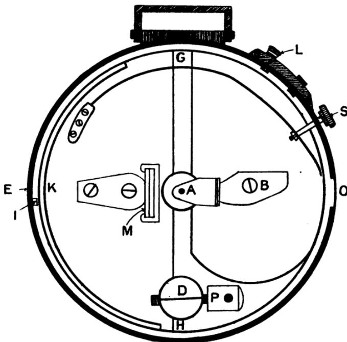
FIG. 5.—WATKIN MIRROR CLINOMETER (INTERIOR)
