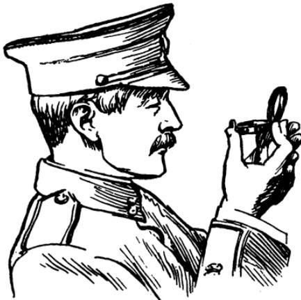
FIG. 15.—OBSERVING A BEARING WITH THE MAGNETIC COMPASS
