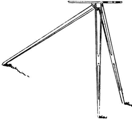
FIG. 7.—PLANE-TABLE ON A SLOPE
