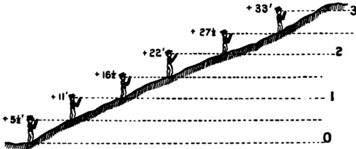
FIG. 28.—CONTOURING WITHOUT INSTRUMENTS
