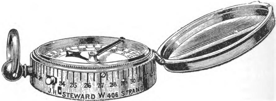
FIG. 35.—MAGNETIC LUMINOUS COMPASS (N.C.O.'S PATTERN)
