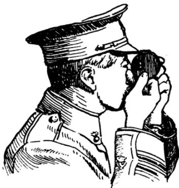
FIG. 6.—THE MIRROR CLINOMETER IN USE
