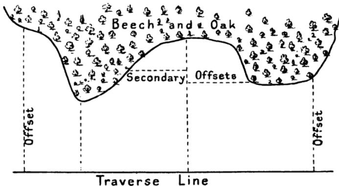
FIG. 9.—THE METHOD OF OFFSETS
