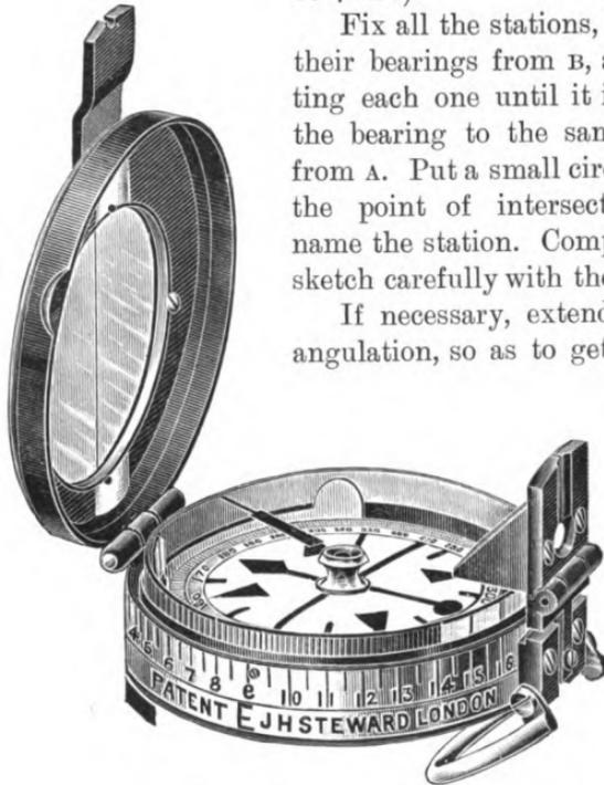
FIG. 18.—LUMINOUS PRISMATIC COMPASS
