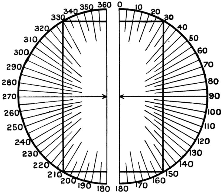
FIG. 17.—THE FORMATION OF A PROTRACTOR FROM A COMPASS-CARD
