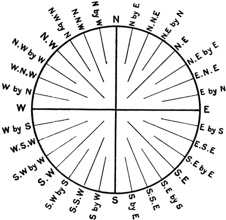
FIG. 10.—THE POINTS OF THE COMPASS
