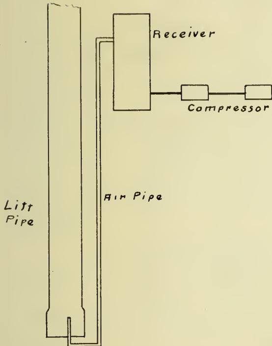
The accompanying figure illustrates a compressor, receiver air and lift pipe as usually operated in deep wells, in which the pressure in the air pipe must be greater than the hydrostatic pressure of the water at the bottom of the pipe, and in quantities sufficient to make the ascending column of air and water in the flow pipe lighter in its total height than
