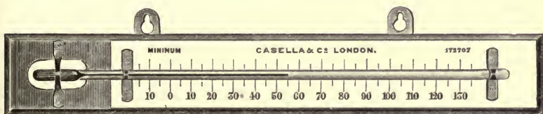
FIG. 5.—RUTHERFORD'S MINIMUM THERMOMETER, FILLED WITH PURE ALCOHOL FOR ORDINARY REGISTRATION, ENGINE-DIVIDED ON THE STEM.
