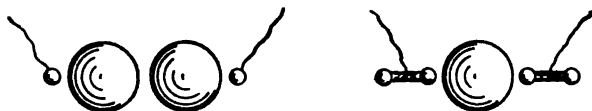
FIGS. 24 and 25.—Two forms of Lodge's oscillator. In the former the oscillations play across between the two middle spheres; in the latter, they surge, like tidal waves, over the surface of the large sphere.
