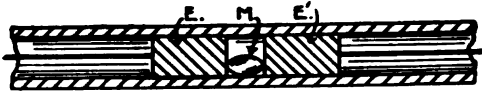
FIG. 95.—Italian navy coherer. E, E' are iron or carbon electrodes, and M a globule of mercury.
