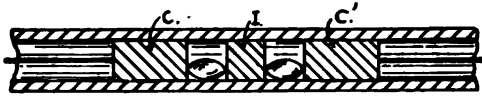
FIG. 96.—Italian navy coherer—second form. The electrodes, C C', are both of carbon, and I is an iron cylinder separating two globules of mercury.
