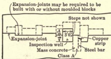
HORIZONTAL SECTION AT EXPANSION-JOINT AT EL.1542
