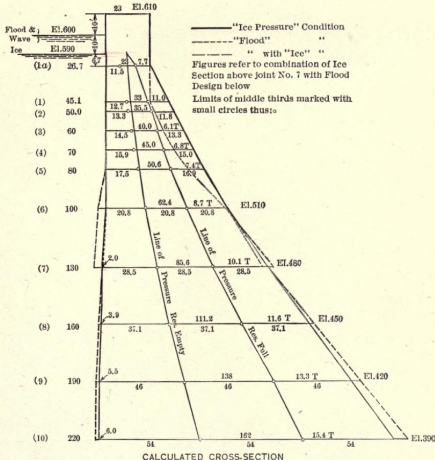
NOTE.—Earth on down-stream toe would not increase compressive stress beyond 20 T. per square foot, if taken at 100 pounds per cubic foot.
