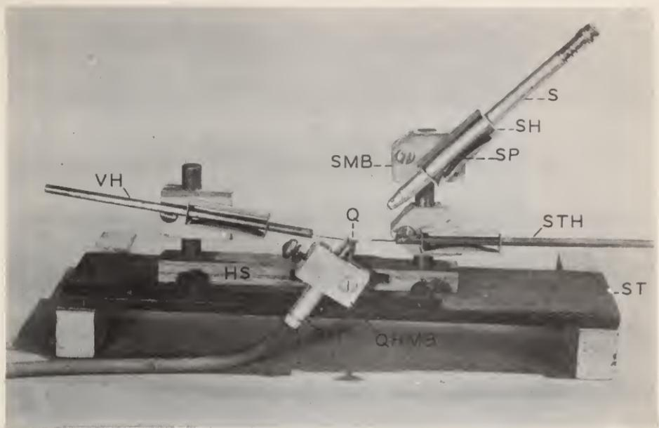
Figure 4.—Manipulating apparatus viewed from operator's side, showing mounting of queen holder, syringe, and holding hooks: HS, Horizontal strip; Q, queen; QH, queen holder; QHMB, queen-holder mounting block; S, syringe; SH, syringe holder; SMB, syringe mounting block; SP, spring; ST, stage; STH, sting hook; VH, ventral hook.
