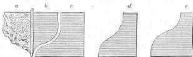
The accompanying diagram shows the three moulds referred to, one of them being *nearly* applied to the finished part of the hull to which it belongs. Thus—(a) represents the unfinished side of the boat; (b) the finished side; (c) is the mould or card cut to correspond with the widest part of the finished side, near the centre of the boat; (d) is the mould for the part near the bow; (e) for that near the stern.
