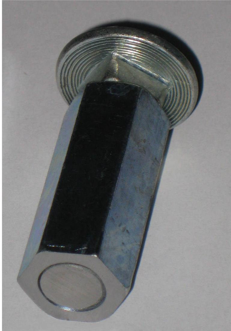
I made the microtome shown above from a long nut (called a union nut) and a carriage bolt. A hex bolt with a flat end would have been better, but the hardware store near me did not have any with threaded ends as long as the union nut. I wanted a long nut, but traditionally homemade microtomes are made with normal size nuts, and they work just fine.
