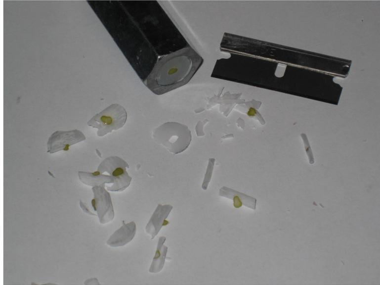
When the wax has hardened, we can use the microtome. With a smooth slicing motion, draw a single edge razor blade across and down over the face of the microtome, keeping pressure against the face, and keeping the very edge of the blade against the metal.
