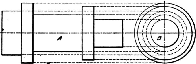
It will be found more necessary to show views of each side (as those at *A* and *C*), as some parts of the form may not be circular, as for instance, a flattened side, a keyway, or any similar special form, that it would be necessary to show.
