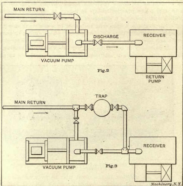
Fig. 2. Method of Connecting Vacuum Pump, used continually, to the Return.
