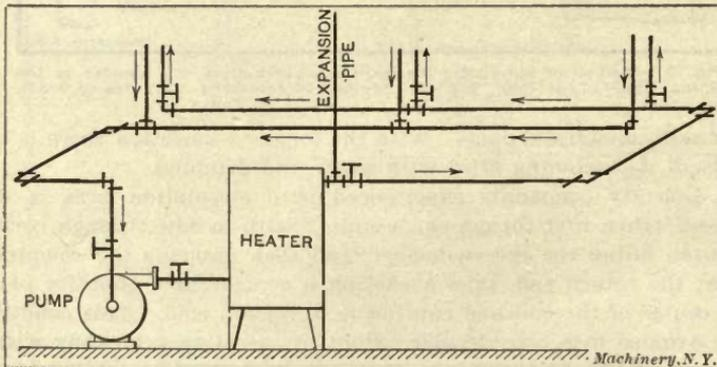
Fig. 19. Two-pipe System for Forced-circulation Hot-water Heating
