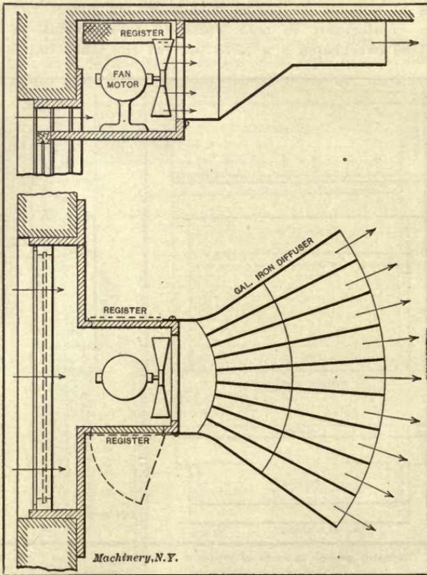
Fig. 37. Simple Arrangement for Desk Fan Ventilation
