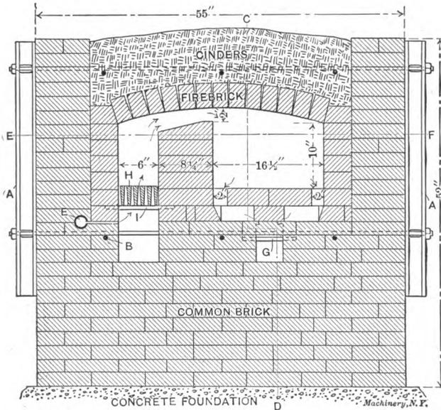
Fig. 8. Case-hardening Furnace. Section in A-B, Fig. 9
