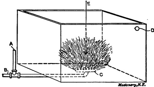
Fig. 15. Hardening Tank Arranged for Mottling and Coloring
