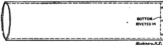
Fig. 13. Gas Pipe used for Packing
