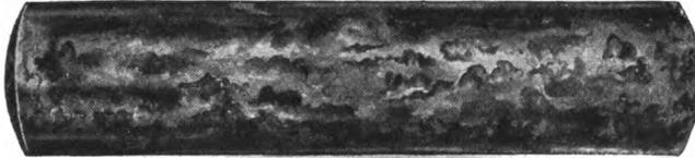
Fig. 17. Sample of Work Case-hardened for Colors
