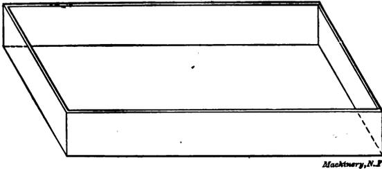
Fig. 12. Suitable Form of Box for Packing Work for Hardening
