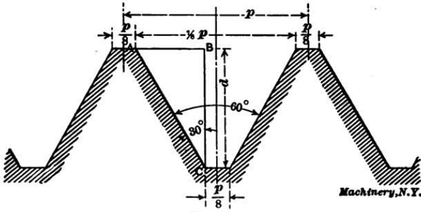
In the illustration,  $p$  is the pitch of the thread. The pitch, of course, equals  $\frac{1}{\text{No. of threads per inch}}$ .\*
