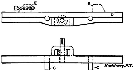
Fig. 17. Support for Rack and Pinion
