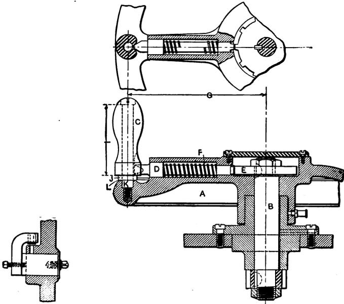
Fig. 12. Jig for Set-screw Holes
