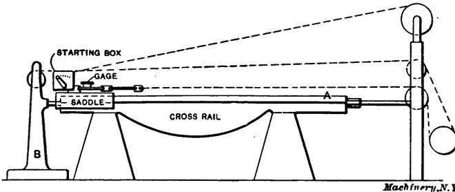
Fig. 25. Pulling Machine, Fig. 23, and Tension Indicator, Fig. 23, in Position for Moving a Planer Saddle along the Cross-rail
