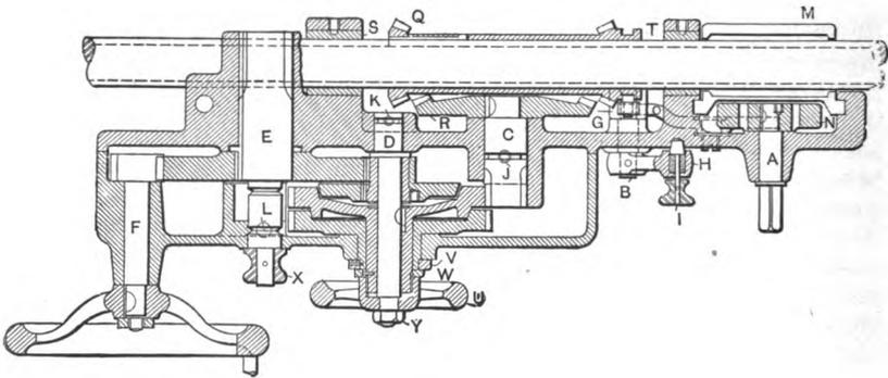
Fig. 9. Engine Lathe Apron to be assembled
