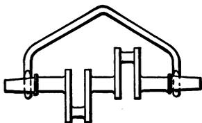
Fig. 28. Machine Steel Sling for Lifting Crank-shafts
