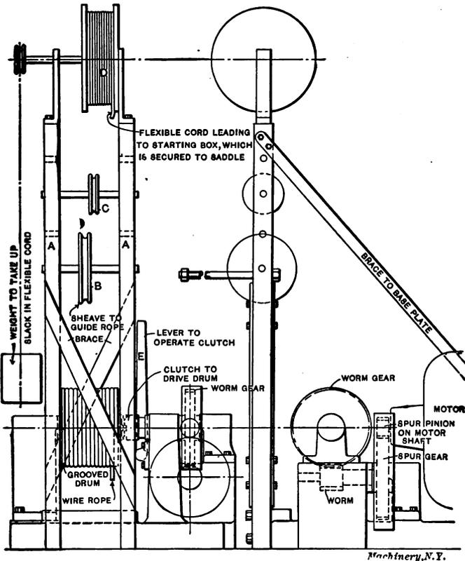
Fig. 22. Pulling Device for Large Planer Saddles
