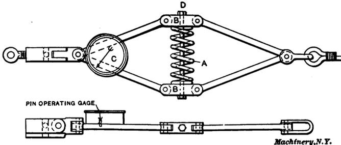
Fig. 23. Indicating Mechanism for Pulling Device
