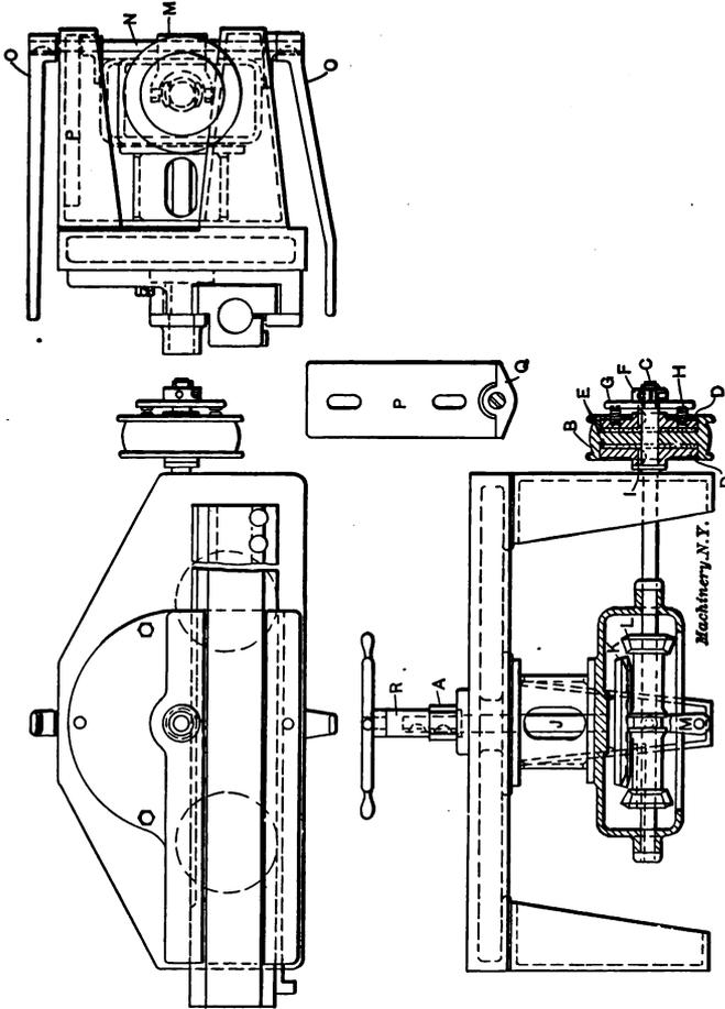
Fig. 21. Machine for Imparting Motion to Boring Mill Flans while Scraping
