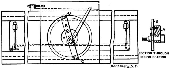
Fig. 20. Rack and Pinion for Pulling a Planer Saddle
