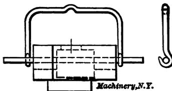
Fig. 29. Device for Lifting Turrets
