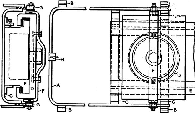
Fig. 38. Device used when fitting a Saddle to a Cross-rail
