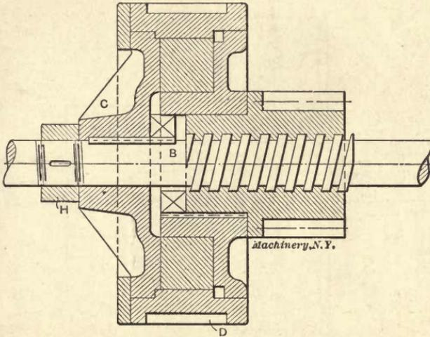
Fig. 13. Automatic Screw Brake for Overhead Electric Cranes
