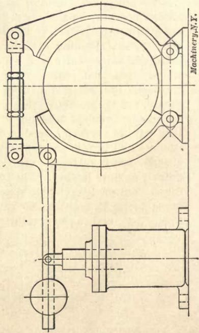
Fig. 11. Typical Design of Compact Clamp Brake for Electric Cranes
