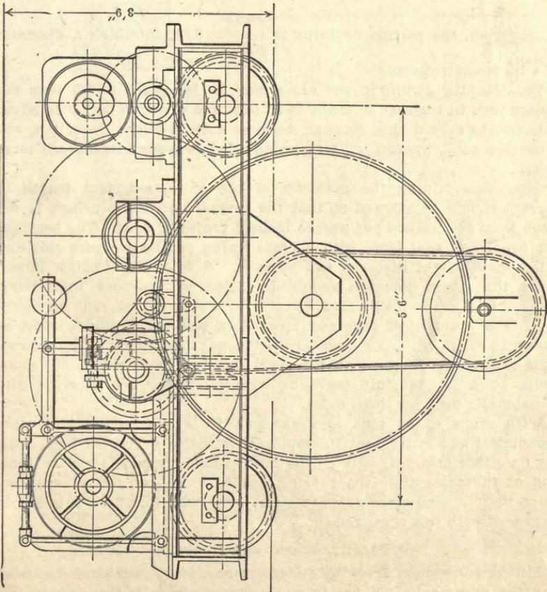
Fig. 4. Crab for 20-ton Three-motor Electric Overhead Crane with Steel Frame
