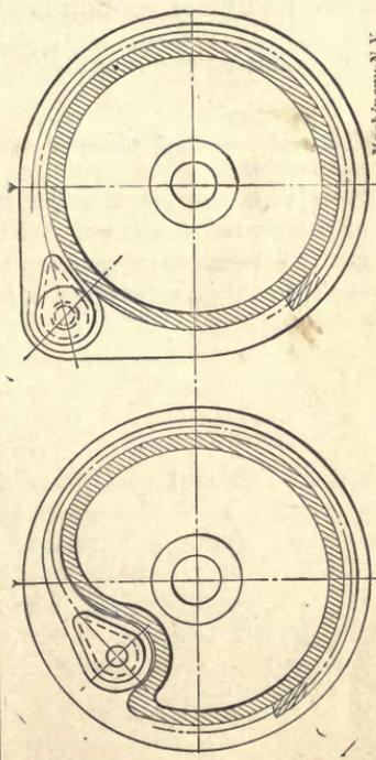
Fig. 7. Two Methods in use for Anchoring the Lifting Ropes Machinery, N.Y.
