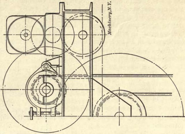
Fig. 5. Crab, similar to the one shown in Fig. 4, slightly altered to accommodate Auxiliary Barrel for Light Loads
