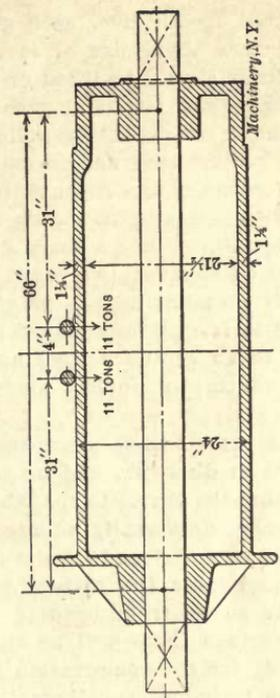
Fig. 8. Barrel for a 40-ton Overhead Electric Crane Machinery, N.Y.
