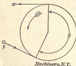
$\mu$  = coefficient of friction = 0.2 for iron to iron, 0.3 for wood to iron, 0.4 for leather to iron.  $P$  = pull on brake rim.  $x$  = strain on loose end of brake strap.  $F$  = strain on fast end.  $\theta$  = arc embraced by strap (in degrees). Table gives tension on brake straps when  $P = 1$ .
