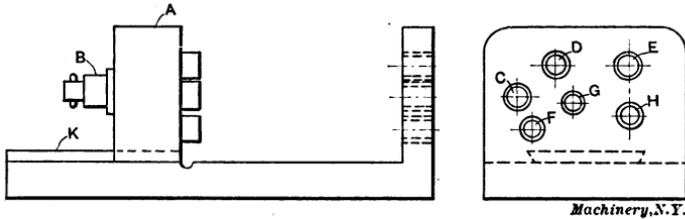
Fig. 124. Principle of Multiple Bar Boring Jig
