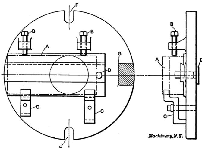
Fig. 184. Fixture for Recessing Work shown in Fig. 182
