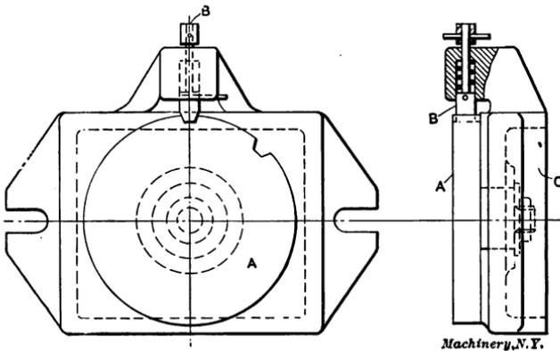
Fig. 186. Another Type of Indexing Fixture
