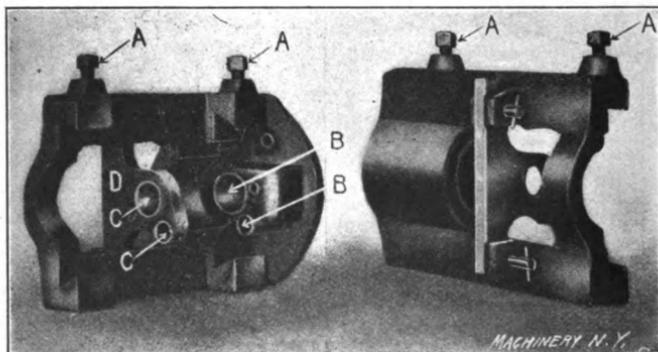
Fig. 126. Example of Small Boring Jig, with Removable Leaf for Holding Guide Bushings
