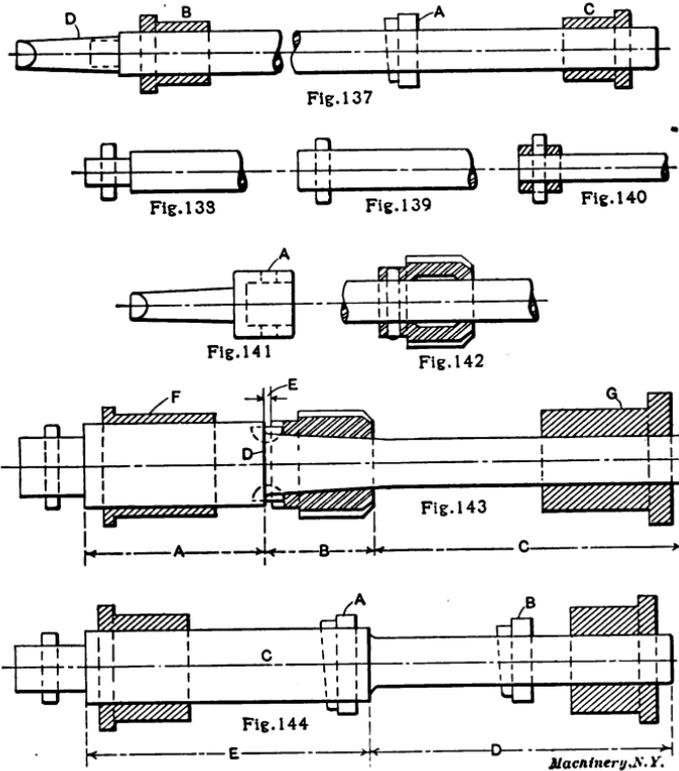
Figs. 137 to 144. Boring Bars of Different Types
