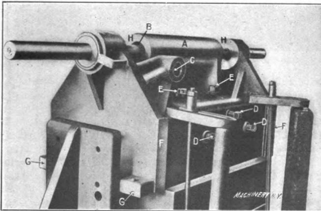
Fig. 128. Common Type of Medium Size Boring Jig
