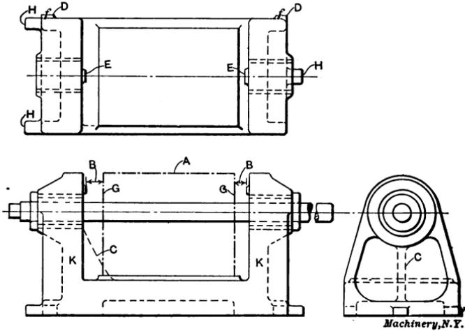
Fig. 109. General Outline of Simple Boring Jig
