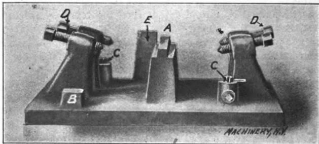
Fig. 180. Simple Type of Milling Fixture
