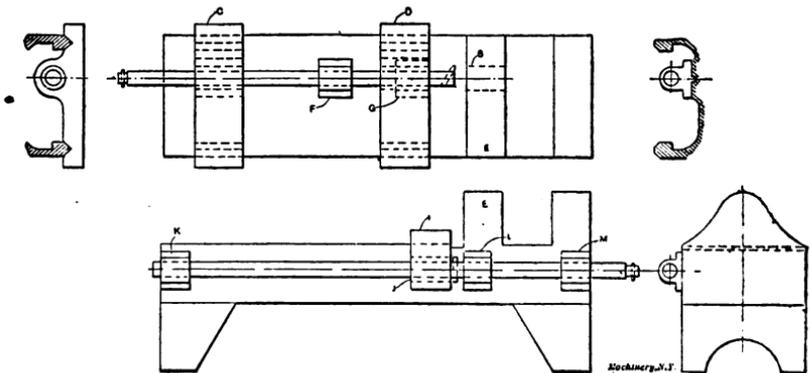
Fig. 134. Examples of Boring where Parts of the Machine being Built are Used as Guiding Means
