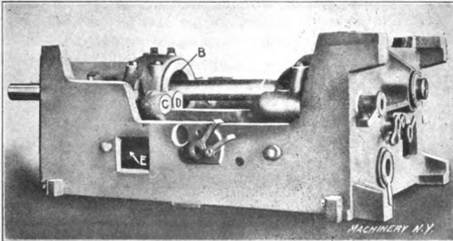
Fig. 136. Another View of the Jig in Fig. 135. Note that Holes are Drilled or Bored from All Sides
