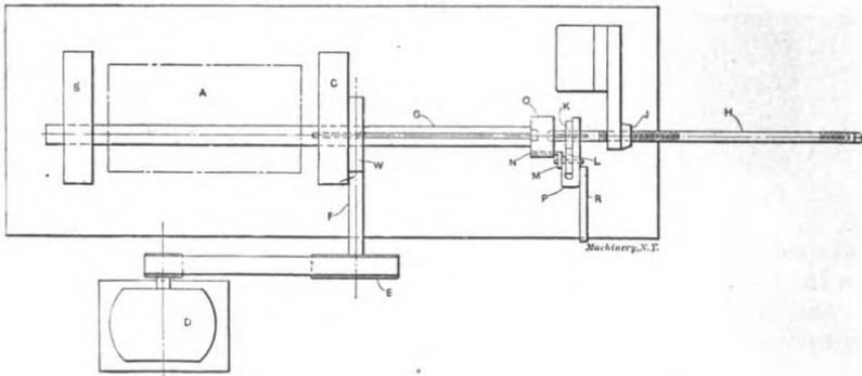
Fig. 132. Outline of Arrangement of the Drive and Feed of the Boring Bar of the Jig in Fig. 131
