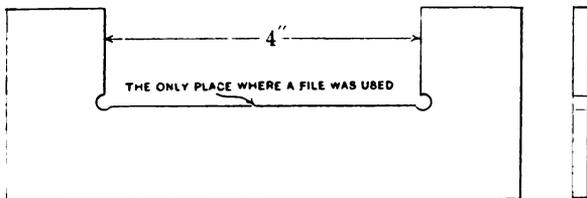
Fig. 7. Snap Gage Ground to Size on Disk Grinder.
