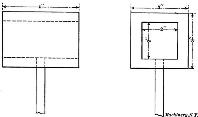
Fig. 9. Hollow Cast Iron Block used for Test.
