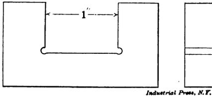
Fig. 5. Snap Gage Finished on Disk Grinder.
