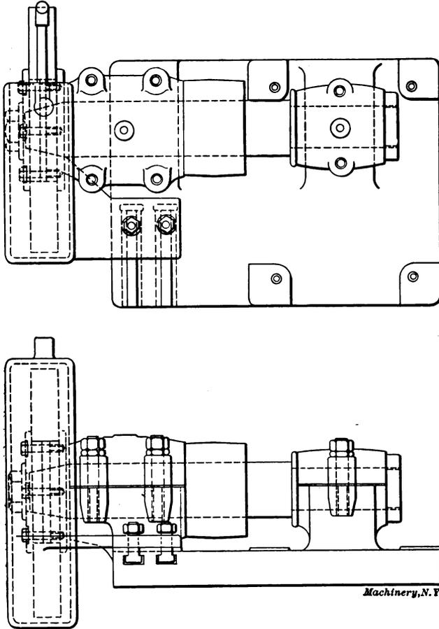
Fig. 2. Grinding Head for External Grinding Machine.
