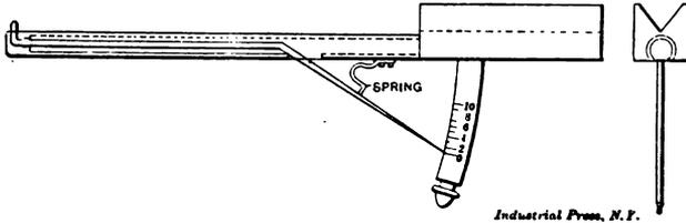
Fig. 64. Indicator for Testing Truth of Holes.
