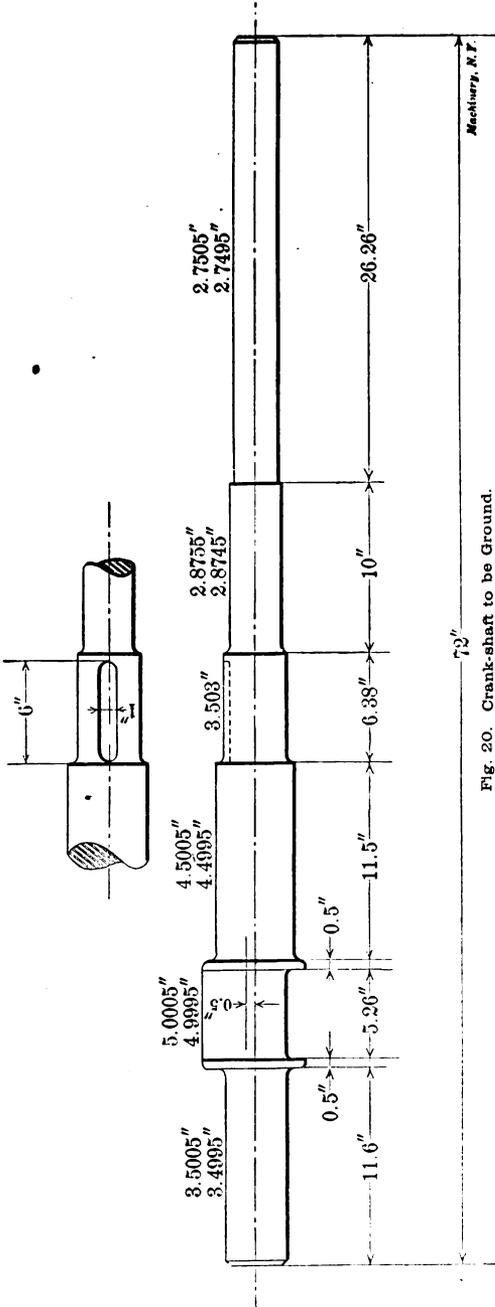
Fig. 20. Crank-shaft to be Ground.
