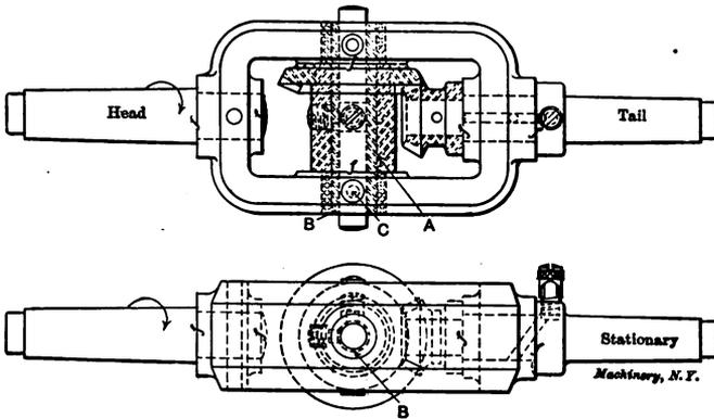
Fig. 52. Fixture for Grinding Spherical End Measure Rods.
