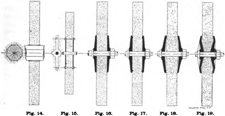
worthy of notice that in nearly every instance the cracks radiated from points where the lead bushing projected into the body of the wheel.
