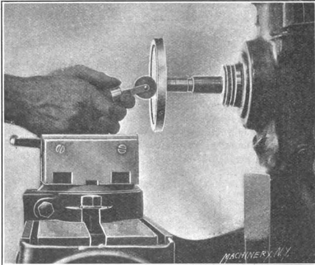
Fig. 59. Charging the Lap with a Roller.
