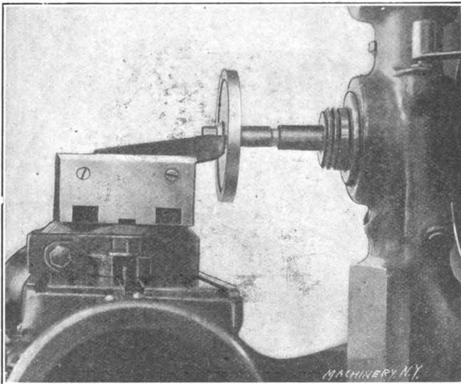
Fig. 58. Truing the Lap with a Tool held in the Vise.
