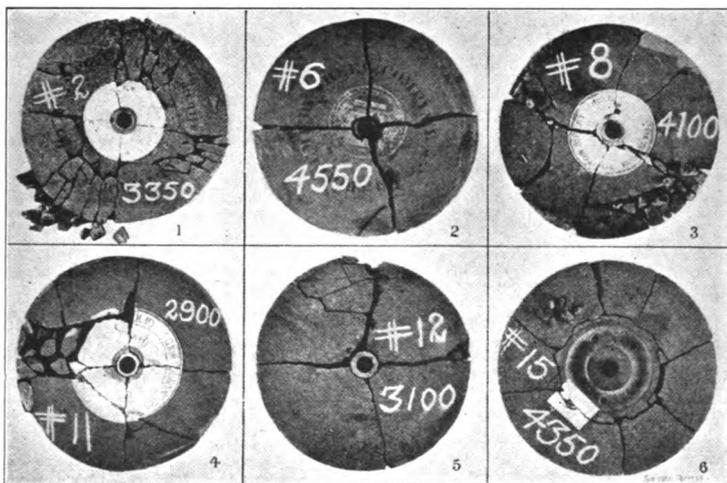
Fig. 13. Various Ways in which Emery Wheels Burst.
