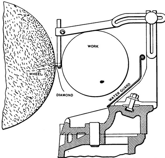
Fig. 1. Fixture for Truing Emery Wheel with Diamond. *Machinery, N.Y.*
