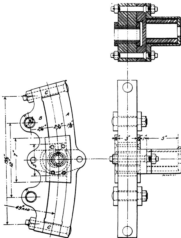
Fig. 21. Wrought Iron Case-hardened Link for Consolidation Locomotive
