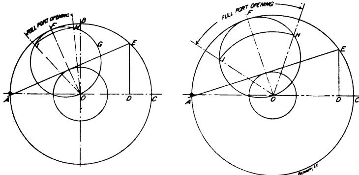
Fig. 13. Valve Diagram for Atlantic Type Locomotive
