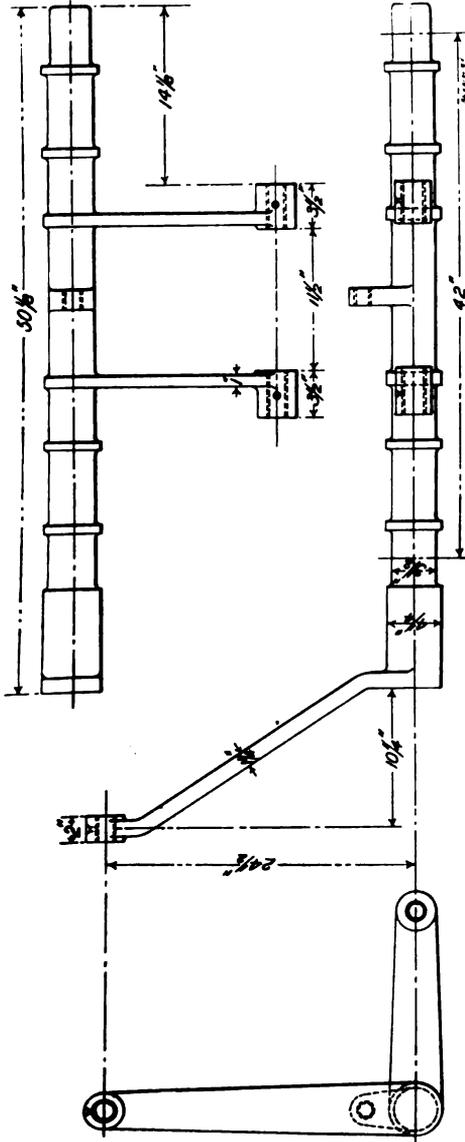
Fig. 28. Lifting Shaft for Consolidation Locomotive
