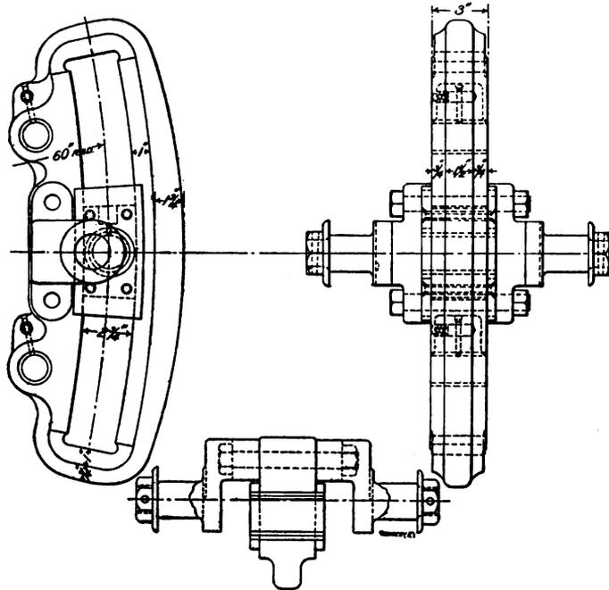
Fig. 22. Cast Steel Link for Atlantic Type Locomotive
