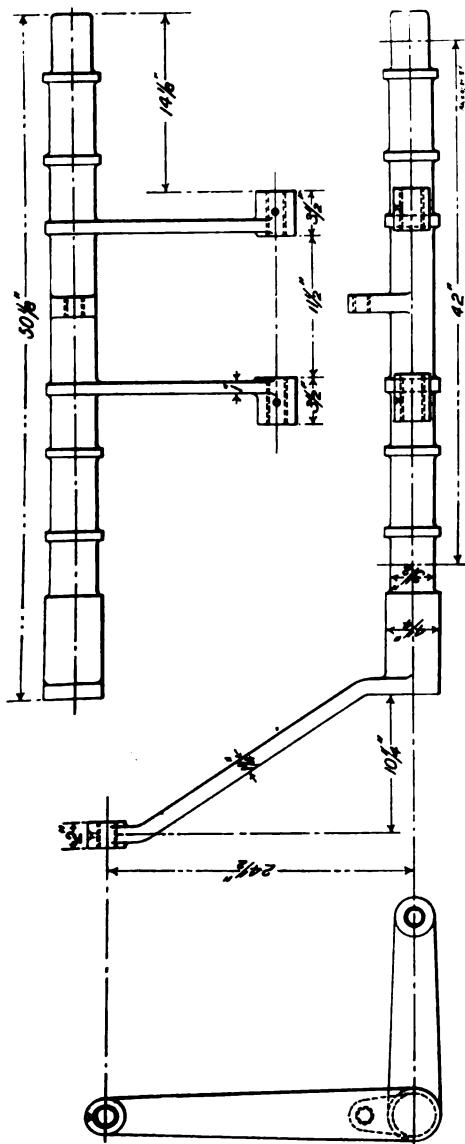
Fig. 23. Lifting Shaft for Consolidation Locomotive
