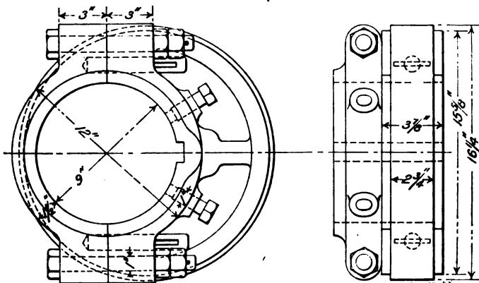
Fig. 18. Eccentric for Consolidation and Atlantic Type Locomotives
