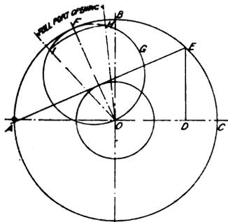
Fig. 13. Valve Diagram for Atlantic Type Locomotive
