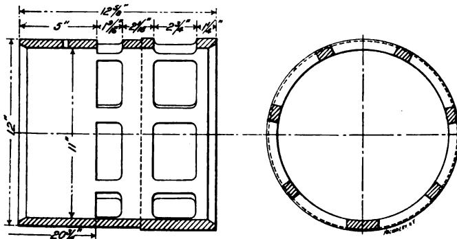
Fig. 11. Valve Chest Bushing for Atlantic Type Locomotive
