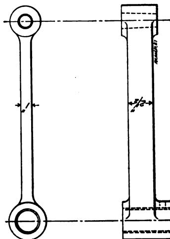
Fig. 24. Link Hanger for Consolidation Locomotive
