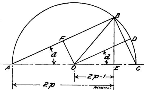
Fig. 3. Diagram for Finding Angular Advance of Eccentric
