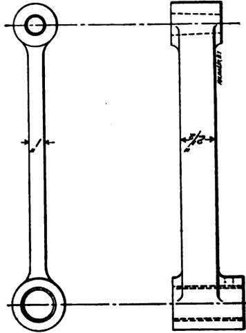
Fig. 24. Link Hanger for Consolidation Locomotive
