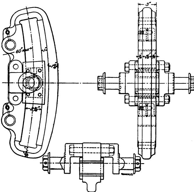
Fig. 22. Cast Steel Link for Atlantic Type Locomotive
