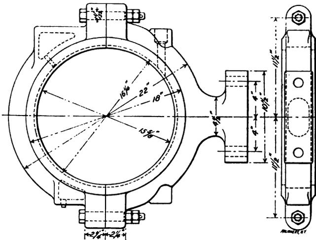
Fig. 19. Eccentric Strap for Consolidation and Atlantic Type Locomotives
