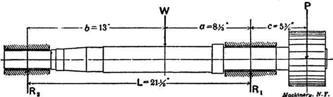
Fig. 10. Dimensions and General Arrangement of Shaft
