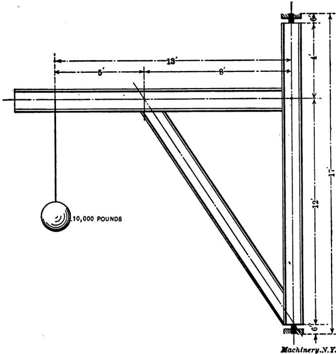
Fig. 8. General Design of Crane in Problem 2
