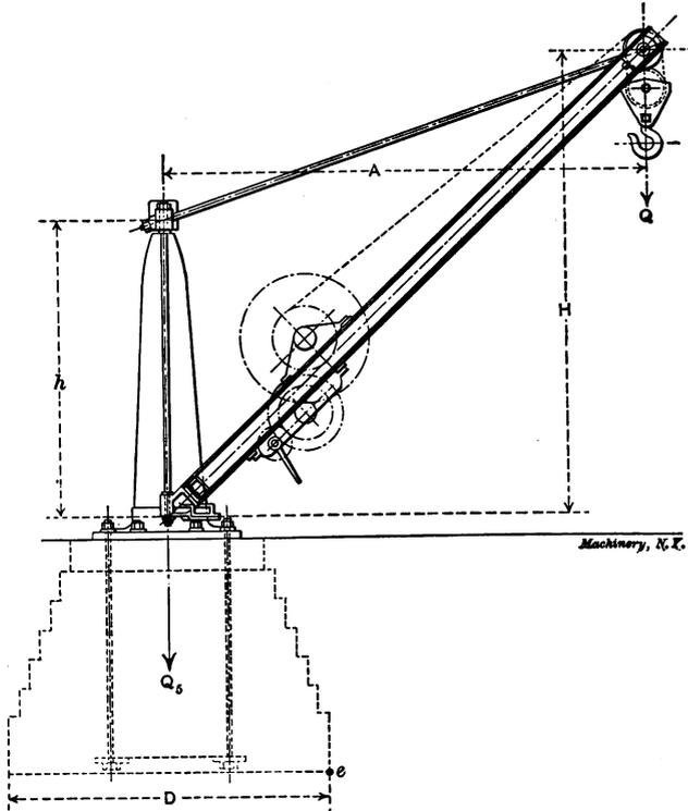
Fig. 16. General Lay-out of Pillar Crane
