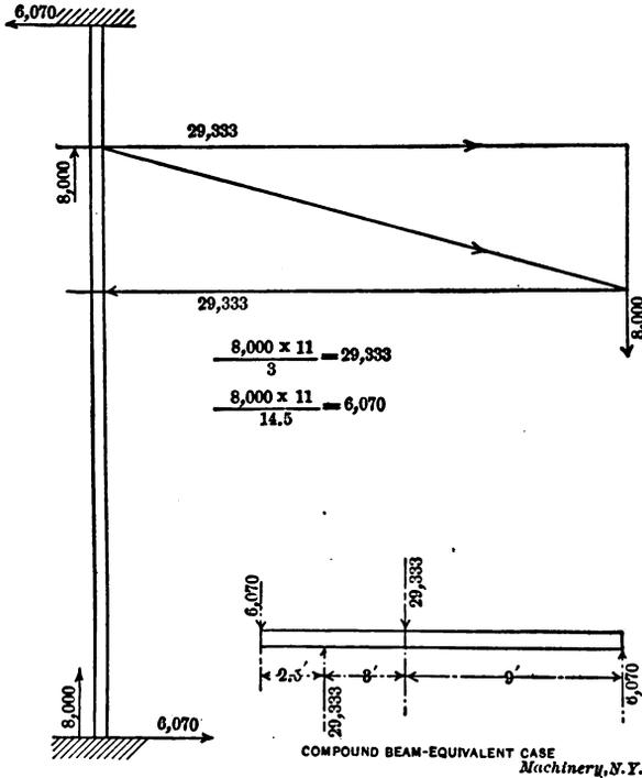
Fig. 6. Forces Acting on Column of Crane
