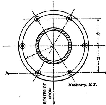
Fig. 19. Lay-out of Arrangement of Flange Bolts
