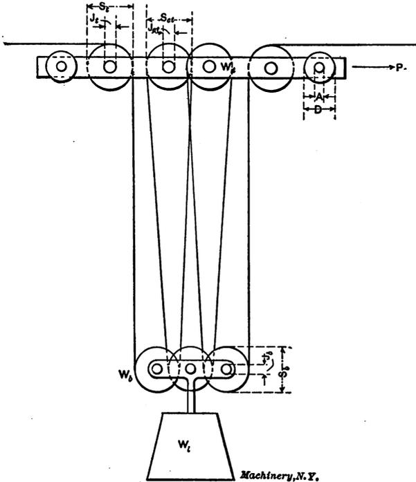
Fig. 16. Trolley with Sheave Suspended by Six Parts of Rope
