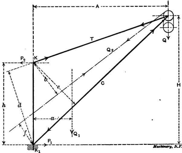
Fig. 17. Diagrammatic View of Pillar Crane
