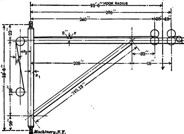
Fig. 3. General Dimensions of Crane to be Designed
