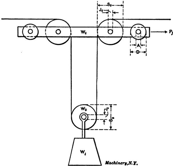
Fig. 13. Trolley with Sheave Suspended by Two Parts of Rope
