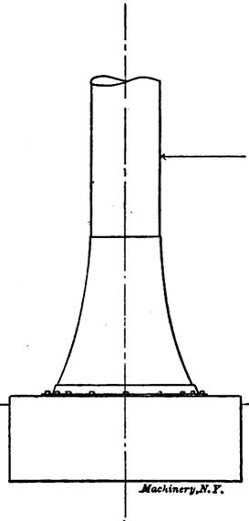
Fig. 9. Wind Pressure Tends to Overturn Chimney.
