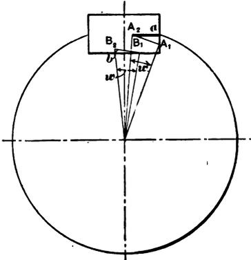
Fig. 26. Diagram of Forces Acting on Key.
