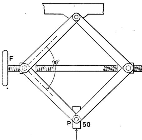
Fig. 35. Double Toggle-Joint.
