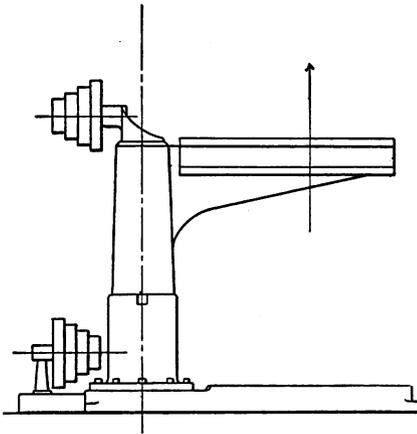
Fig. 8. Radial Drill; Pressure of Feed Tends to Overturn.
