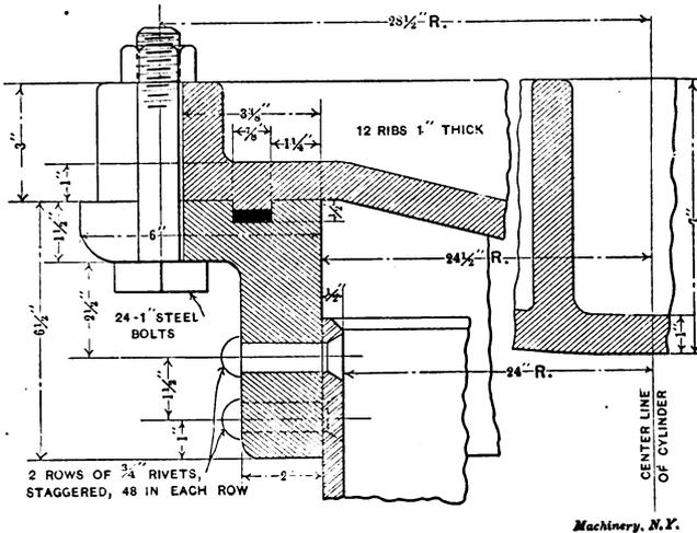
Fig. 20. Design of Mouthpiece Ring and Cover.
