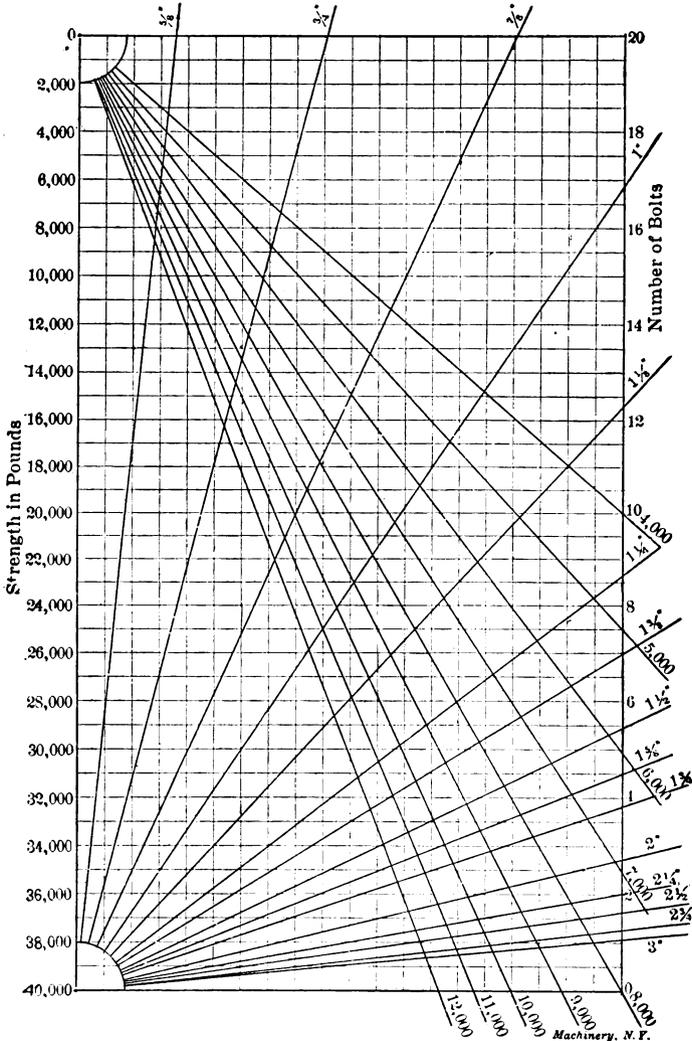
Fig. 5. Diagram of Working Strength of Bolts.
