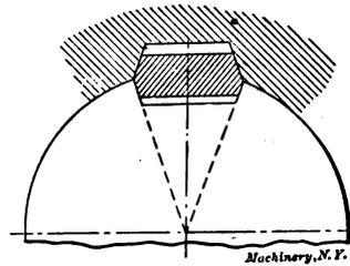
Fig. 27. Proposed Form of Key, Equalizing the Radial and Tangential Pressure.
