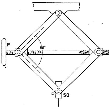
Fig. 35. Double Toggle-Joint.
