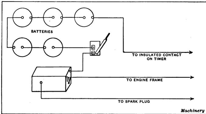
Fig. 7. Wiring for "Jump Spark" with Batteries
