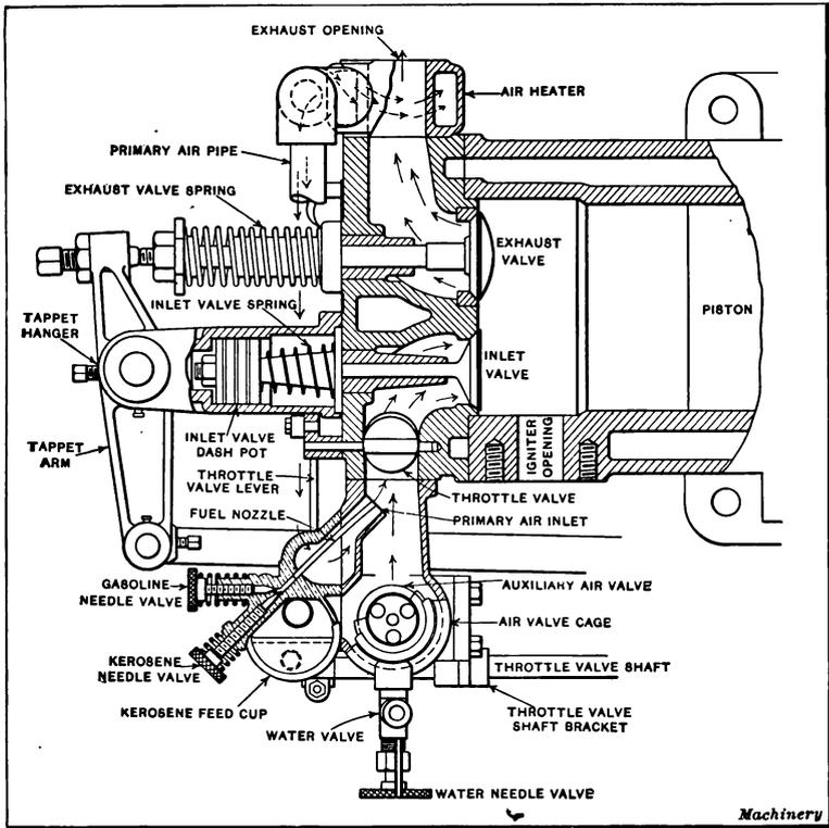
Fig. 5. Sectional View of Oil Engine Cylinder-head
