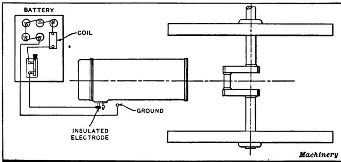
Fig. 9. Wiring for Horizontal Engine with Batteries
