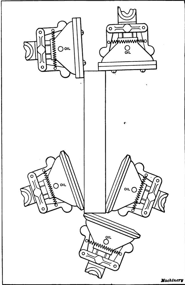
Fig. 14. Diagrammatic View showing the Different Positions that may be used for Driving a Rotary Magneto
