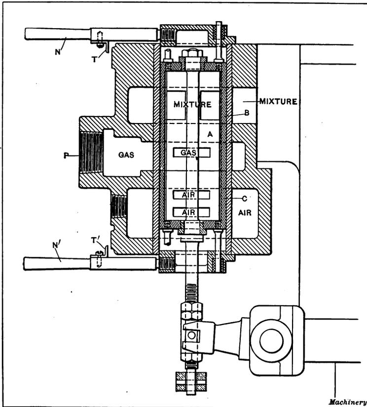
Fig. 6. Mixing Valve used on Westinghouse Gas Engine
