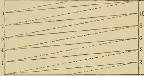
How to get the Lines for Thread of a Worm
