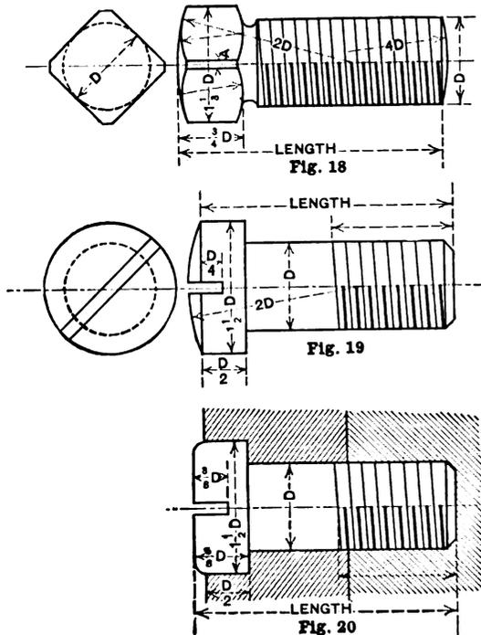
**SET SCREW.** Fig. 18. This has a square head, having its short diameter equal to the diameter of the screw. The construction will be apparent from the figure, on which the proportions are given. The radius for the point of a set screw should be equal to four diameters of the screw.
