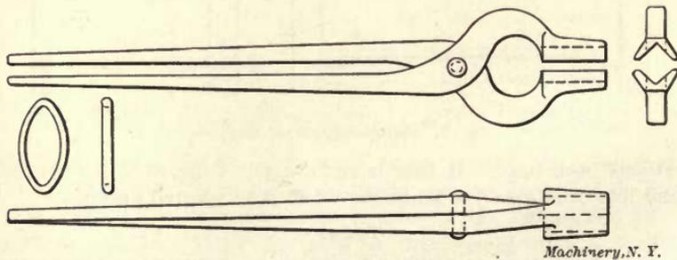
Fig. 9. Tongs with V-shaped Jaws
