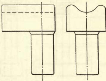
Fig. 3. Correct Form of Bottom Part of Swages
