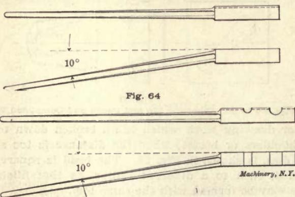
Figs. 64 and 65. Tools used under Steam Hammer for Shearing off Stock
