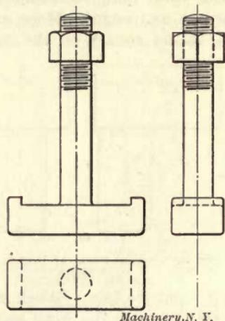
Fig. 6. Clamping Screw Used with Clamp in Fig. 10
