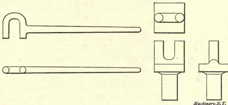
Figs. 17 and 18. Tools for Bending Work
