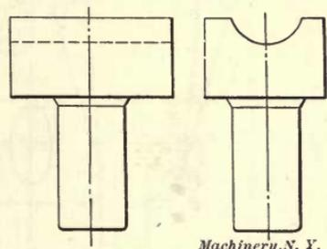
Fig. 4. Incorrect Form of Bottom Part of Swages
