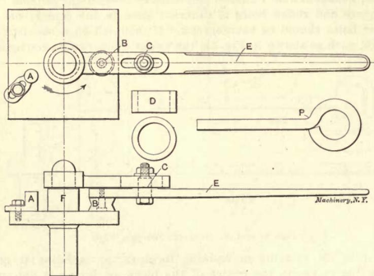
Fig. 19. Tool for Forging Open Eye-bolts or Hooks
