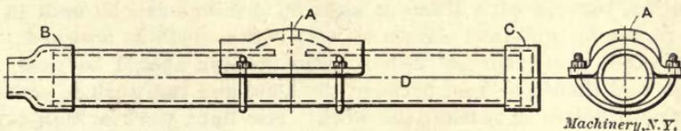
Fig. 29. Air Chamber and Tuyere for Bottom Blast
