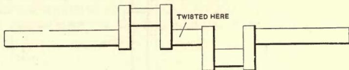
Fig. 13. The Crank-shaft to be Forged
