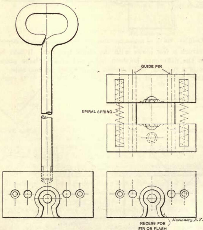
Fig. 59. Dies for Drop Forging under the Steam Hammer
