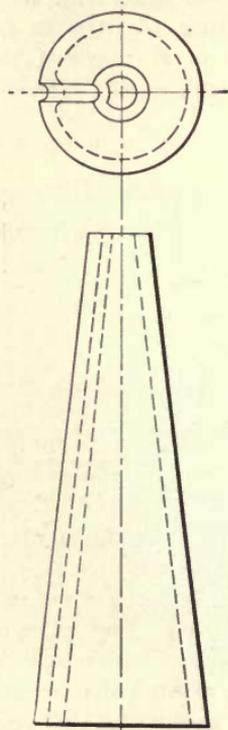
Fig. 15. Taper Cone for Forging Rings, Collars, etc.
