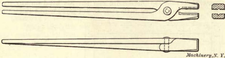
Fig. 8. Approved Type of Tongs with Flat Jaws
