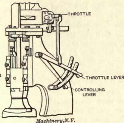
Fig. 34. Improved Arrangement of Throttle Lever
