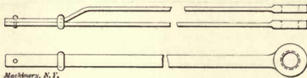
Fig. 52. Swages for Forging Hubs
