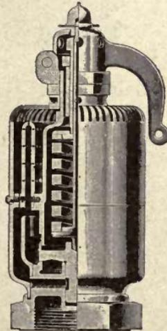
FIG. 11. Sectional View with Lever.
