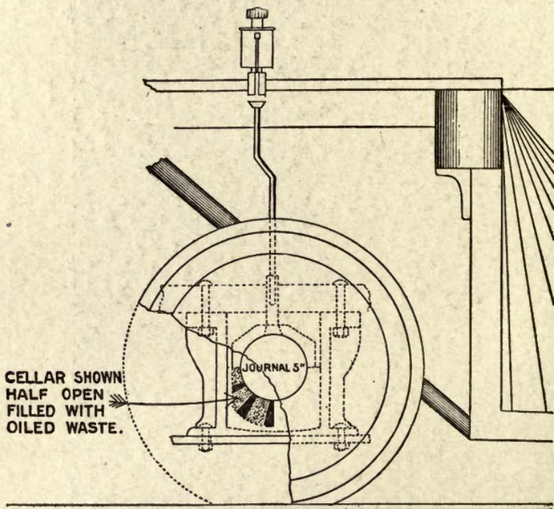
FIG. 1. Acme Engine Truck Cellar and Oil Cup.
