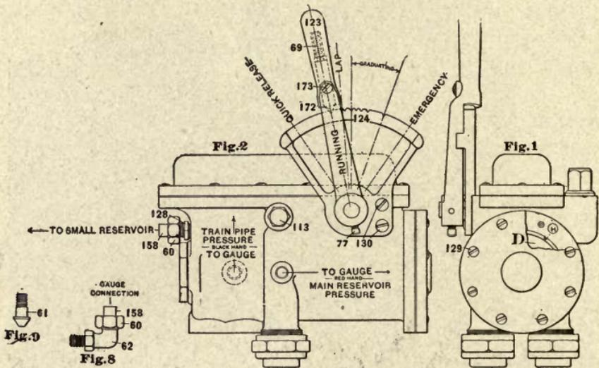
Positive Discharge Engineer's Brake Valve.
