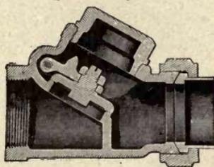
FIG. 1. Swing Intermediate or Line Check.
