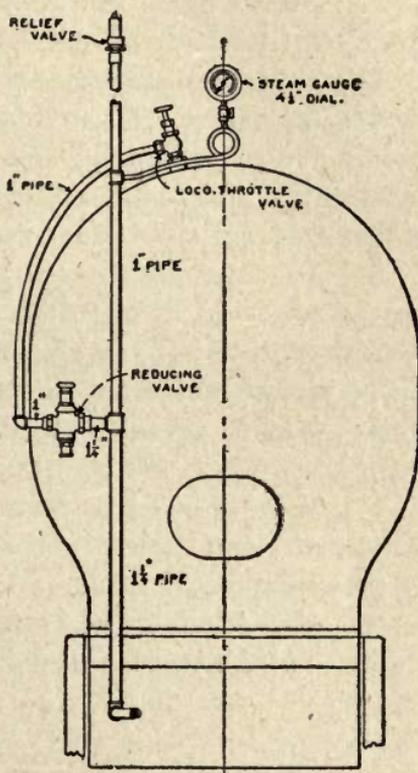
FIG. 8. Location of Steam Heating Cab Attachments.
