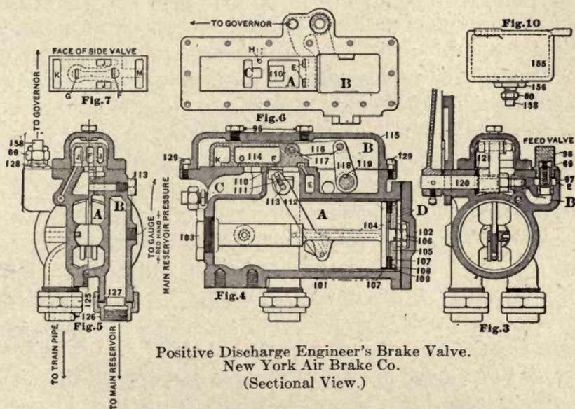
Positive Discharge Engineer's Brake Valve.
