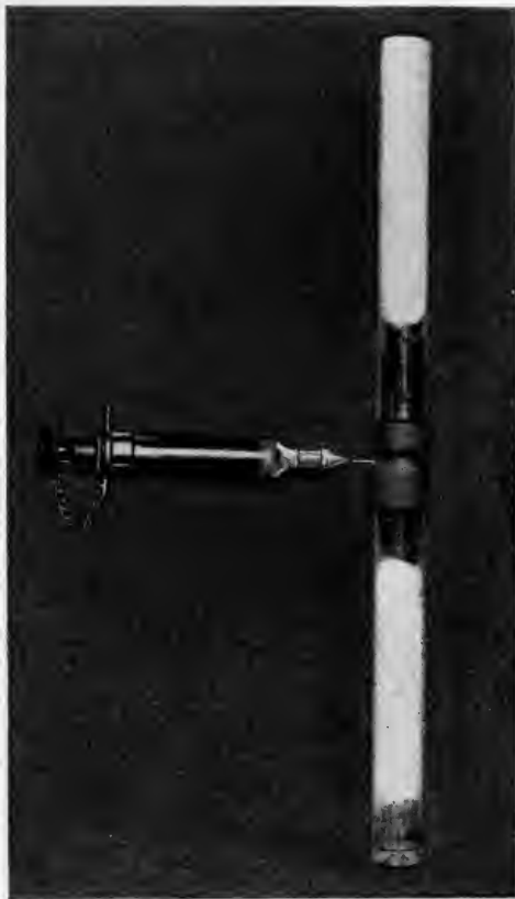
Fig. 123.—Author's simple device for testing movements of solutions of different specific gravity when injected one within the other, the injected solution being colored. Consists of two sections of glass tubing connected by a short section of rubber tubing.
