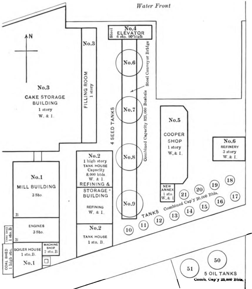
FIG. 47. — 84-PRESS LINSEED OIL MILL AT TIDEWATER.
