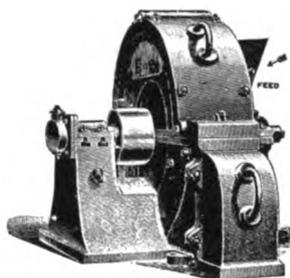
FIG. 61. — COPRA DISINTEGRATOR.
