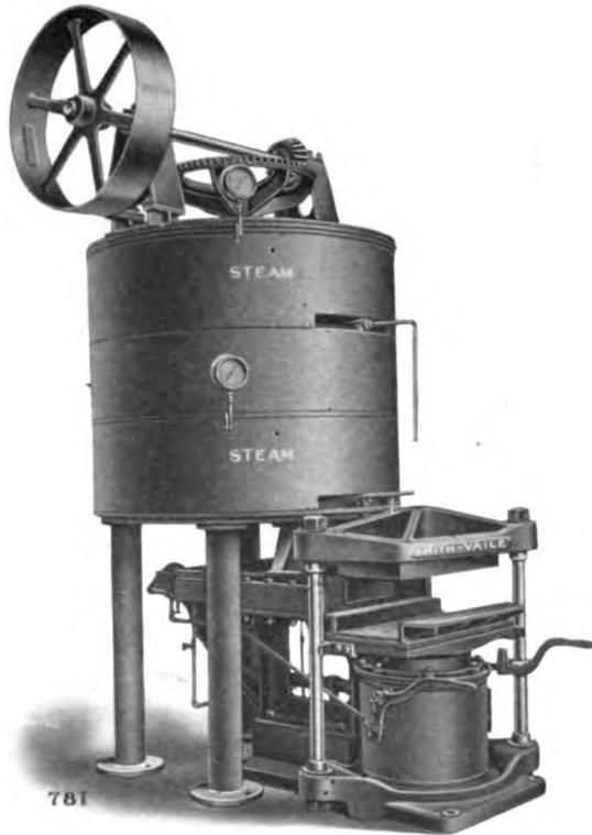
FIG. 18b. — PLATT HEATER AND STEAM FORMER.
