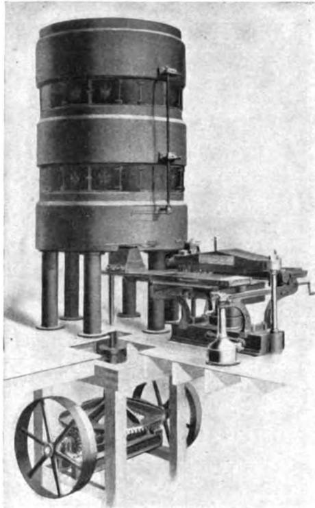
FIG. 15. — BUCKEYE THREE-HIGH 72-INCH LINSEED HEATERS, SHOWING DOUBLE HYDRAULIC CAKE FORMER IN POSITION. SUB-FLOOR DRIVE.
