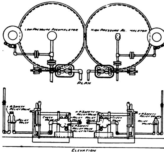
FIG. 29a. — ACCUMULATOR CONTROLLING VALVES AND PIPING.
