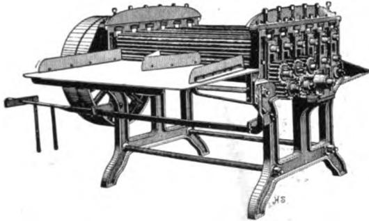
FIG. 53b. — FLAX FIBER BREAKING MACHINE.
