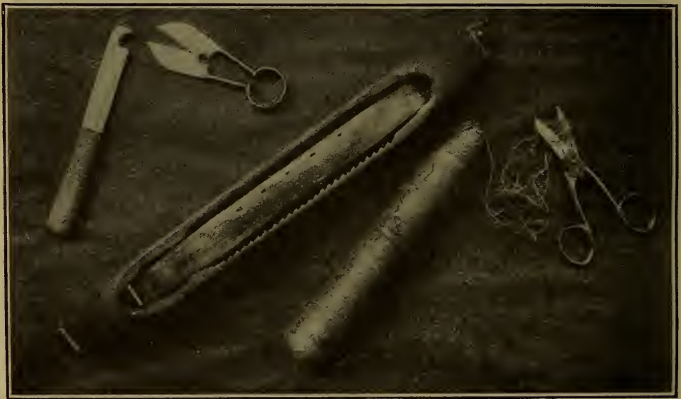
FIG. 9.—Shuttle used in jute weaving and weaver's reed hook, etc.
