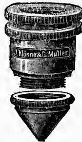
FIG. 29.—Klönne and Müller's Object Marker.
