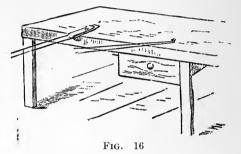
SHOWS THE METHOD USED IN WAXING TEST THREADS.
