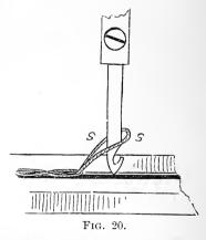
THE NEEDLE IMMEDIATELY AFTER IT HAS CAST OFF A LOOP AND IS RETURNING TO TAKE UP ANOTHER.
