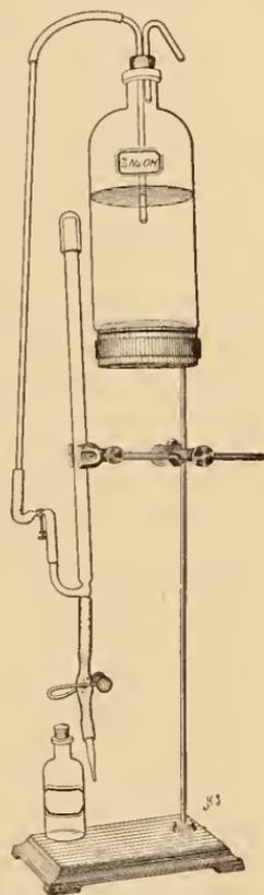
FIG. 1.—Titration apparatus for determining acidity of milk.
