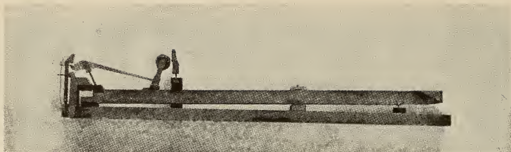
1.—Model of a German or Viennese piano action.
