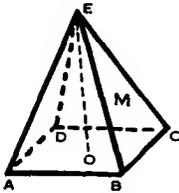
To find the *volume* of a *pyramid* multiply the area of its base by  $\frac{1}{3}$  of its altitude.
