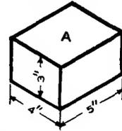
To find the *volume* of any *prism* multiply the area of its base by the height.
