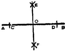
With  $O$  as a center, and any radius, draw arcs cutting at  $C$  and  $D$ .
