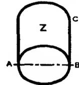
*Example:* Area of curved surface of cylinder *Z* equals the circumference or perimeter of *AB* multiplied by *BC*, the height of the cylinder.
