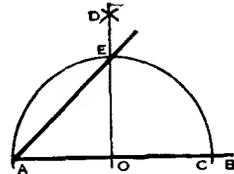
To construct an angle equal to another angle.
