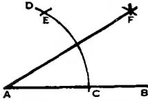
To construct an angle of 45 degrees.
