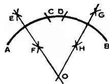
With  $A$  and  $B$  as centers, draw arcs cutting at  $C$  and  $D$ .
