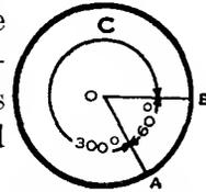
*Example:* Circle *C* contains 360 degrees ( $360^\circ$ ). Angle *AOB* contains  $60/360$  of the whole circle or  $60^\circ$ .
