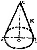
To find the *area* of the slanting surface of a *cone* multiply the distance around its base or its perimeter by  $1/2$  of its *slant height*.
