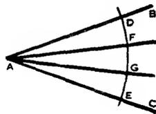
To divide a straight line into any number of equal parts.
