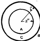
To find the *area* of a *circular ring*, find the area of both the inner and outer circles and subtract the smaller from the larger.
