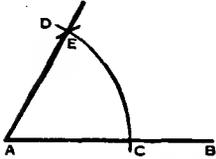
To construct an angle of 30 degrees.
