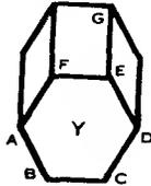
Volume of hexagonal prism *Y* equals the area of hexagon *ABCDEF* multiplied by its height *EG*.
