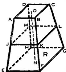
*Example:* Volume of frustum *R* equals area of *ABCD* plus area of *EFGH* plus 4 times area of *JKLM* times  $1/6$  of *ON*.
