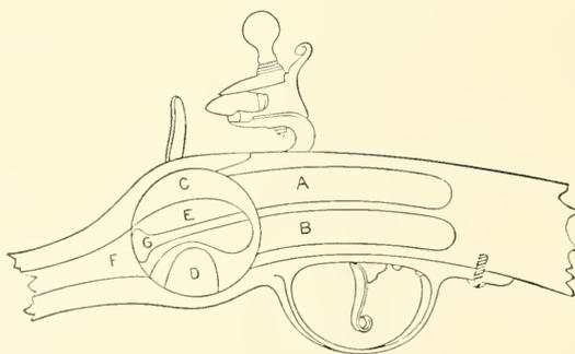
These compartments connect by cylindrical passages with the central chamber in the frame, in which is located a solid cylindrical block (c) with its axis from right to left.
