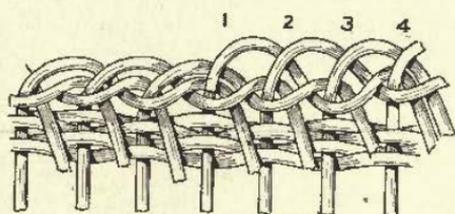
FIG. 119. DETAIL OF CLOSED BORDER NO. 2.
