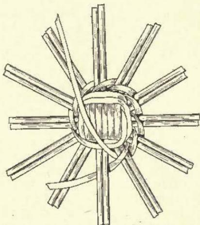
FIG. 128. ROUND BASE WITH SPOKES IN PAIRS.
