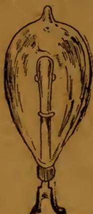
Figure 4 represents a lamp of that kind of 2-candle power, i. e., will give as much light as two ordinary tallow candles. The current necessary to cause the carbon to become white heat, and thus give light, is 2 Volts (3 cells of Grenet battery.) Lamps of this kind are now made varying in candle power from 1-4 to 16 and 20. The 16-candle lamp is the one generally used to light store-rooms with, as this light is not so strong and does not affect the eyesight so much as the arc light.
