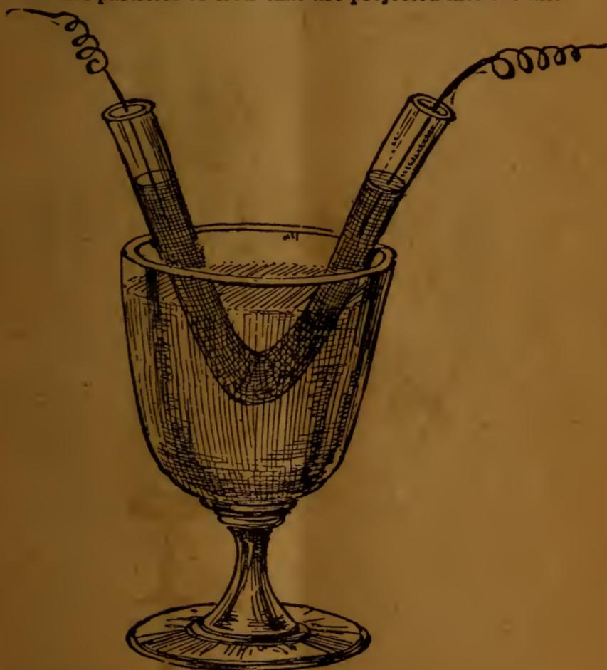
For the following experiment a V-shaped tube is necessary, which may be made by beating an ordinary glass tube in a Bunsen or oxy-hydrogen flame, and bending when it has acquired a cherry colored heat.
