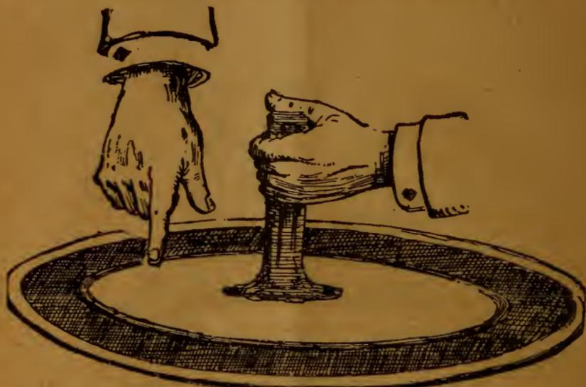
tricity on the vulcanite, the † electricity of the disk is now free, and if a knuckle of one of your hands (Fig. 2) is brought near it, a bright spark will pass from it to your hand, and it will become discharged.
