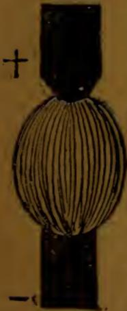
stopped. The carbon of the  $\dagger$  pole becomes volatilized, and the light-giving particles are transported from the  $\dagger$  pole to the  $-$  pole, forming a bridge of luminous vapor between the poles. What we see is not electricity, but luminous matter. Neither light nor a current can exist without matter, as may be shown by trying to pass a current between two metallic poles, a little way apart, in a charcoal vacuum; no spark can be produced.
