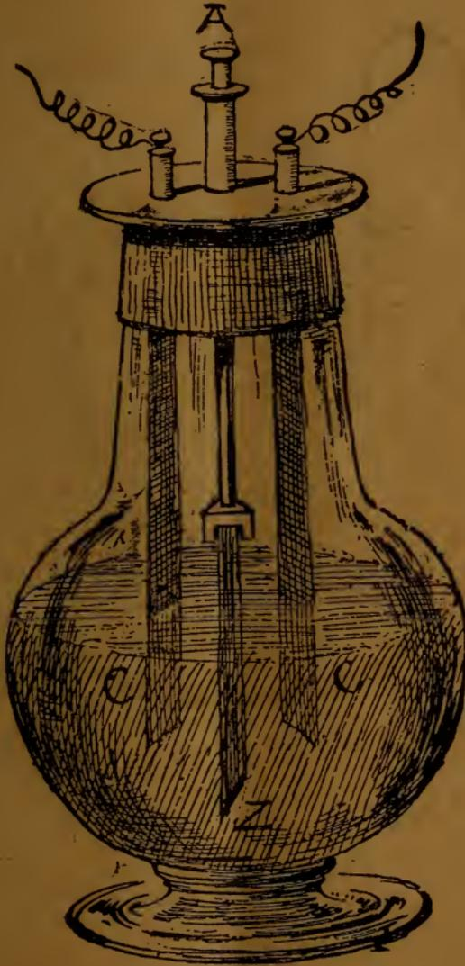
This is the best and most powerful form of battery known. With two cells of this battery, a small two-candle incandescent lamp may be burned for 2 1-2 hours. Eighteen small cells will burn a 6-candle lamp for 1 1-2 hours. Later on I will describe a pocket battery which any boy can make and which will light a
