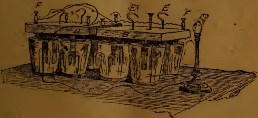
The hooks, E, are fastened to both sides of the top board, and are turned out at right angles to the board, whenever it
