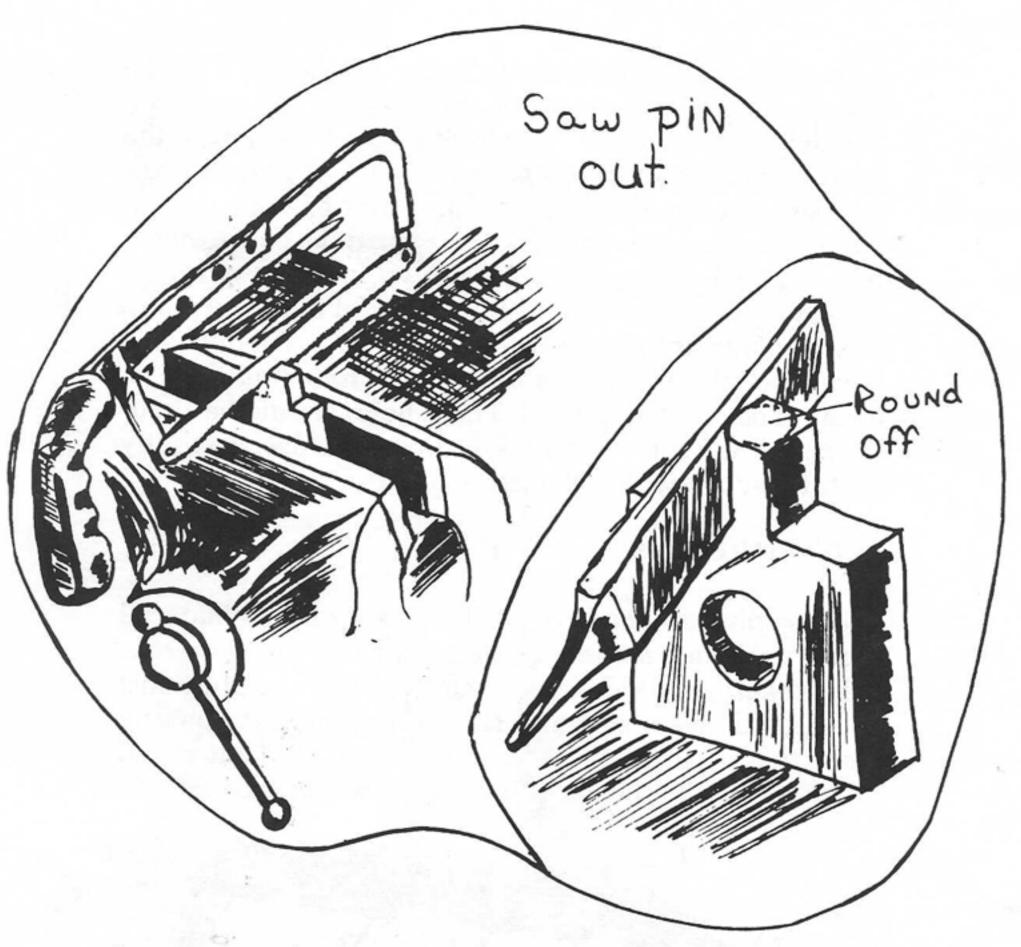
length. Now lay the measurements out the way that the drawing shows, and cut the pin portion out with a hack saw. This will have you a square pin. Place the body portion of the pin in a vice and round off the pin portion with a file as is shown. Next drill a no. 9 hole, or something larger than the diameter of the screw you use, in the dead center of the body portion of the pin. These pins are inlaid into the indexing head as shown and screwed into place.
