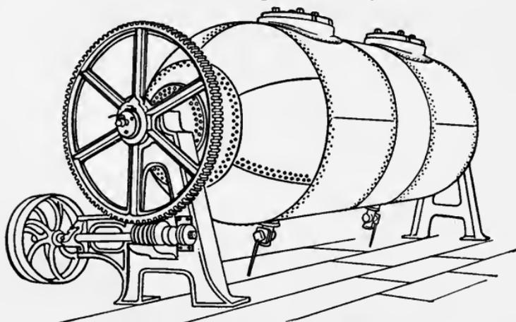
Fig. 2. Revolving Boiler for "cooking" rags.
