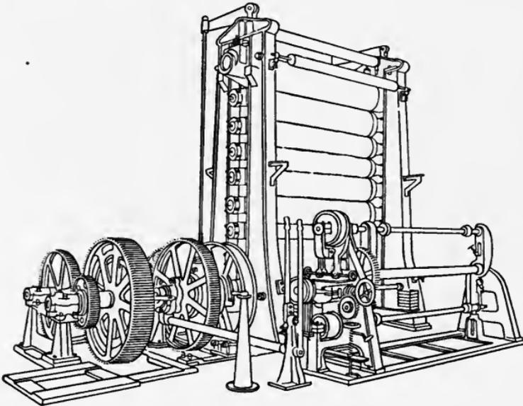
Fig. 8. Stack of calender rolls.
