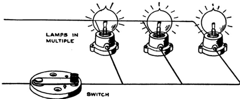
FIG. 159.—Lamps Controlled by One Switch.
