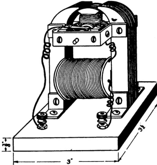
FIG. 133.—The completed Electric Motor.
