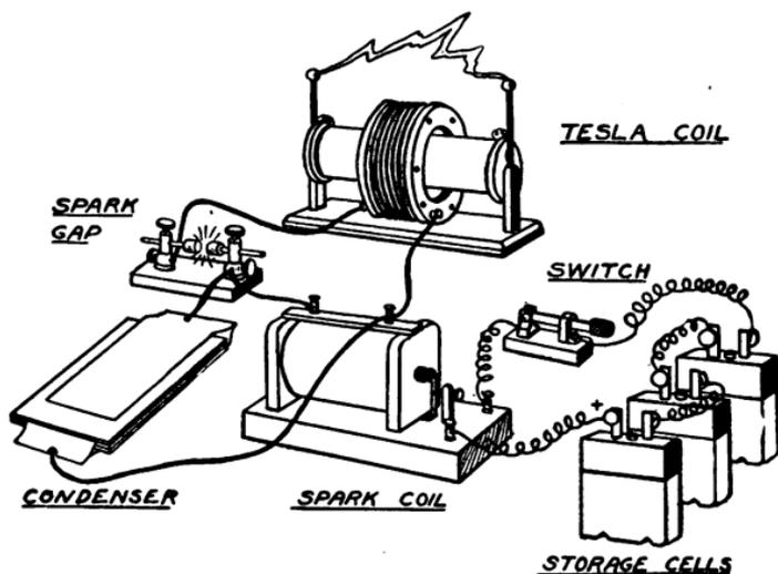
FIG. 177.—Diagram of connections for operating the Coil.
