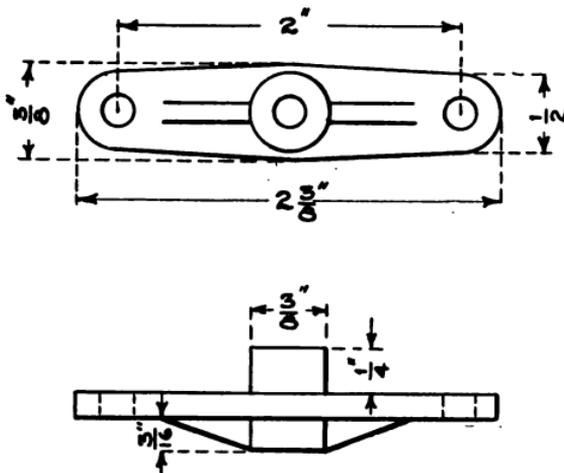
FIG. 129.—Details of the Bearings.
