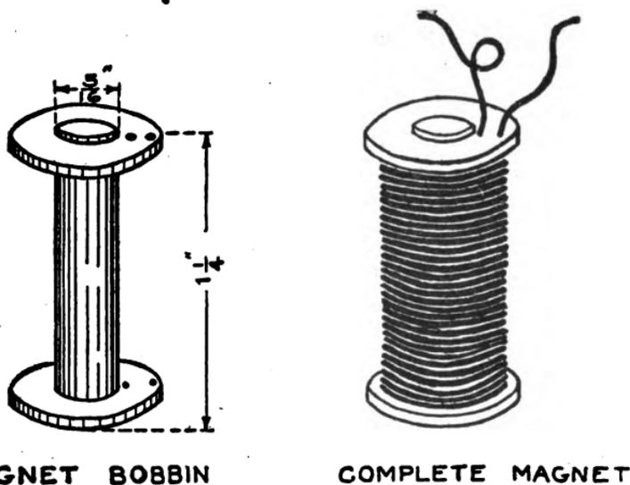
FIG. 85.—The Electro Magnets.
