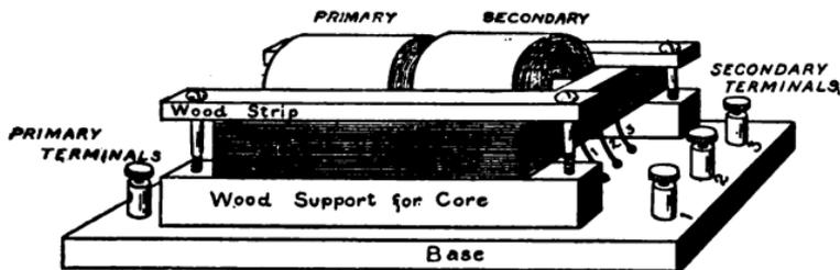
FIG. 63.—The Step-down Transformer mounted on a Wooden Base.
