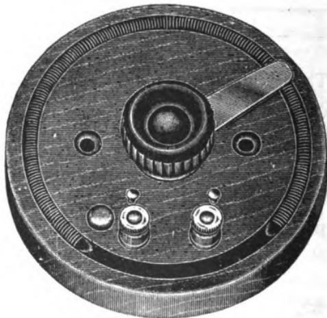
FIG. 82.—The completed Rheostat.
