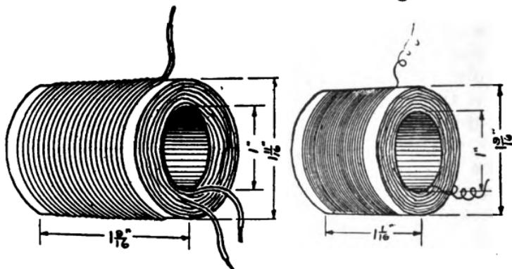
FIG. 61.—Details of the Primary and Secondary Windings.
