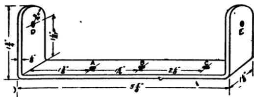
FIG. 146.—Details of the Engine Frame.
