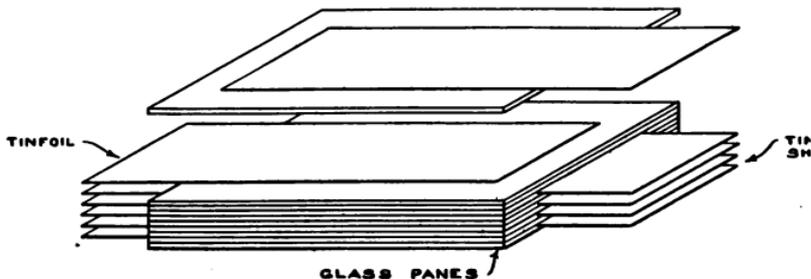
FIG. 178.—Plate Glass Condenser.
