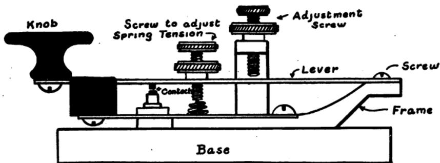
FIG. 89.—Side View of Key.
