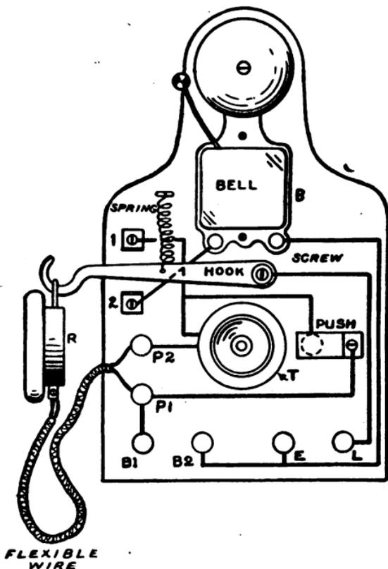
FIG. 94.—The Complete Telephone.
