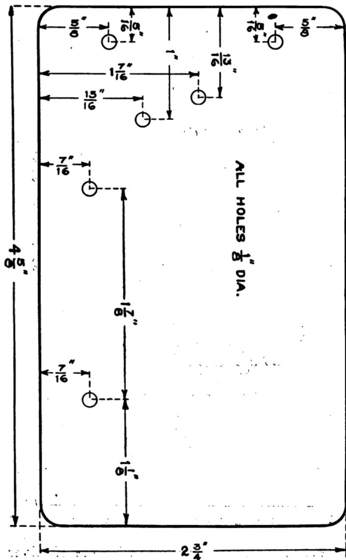
FIG. 103.—The Base with Location of Holes.
