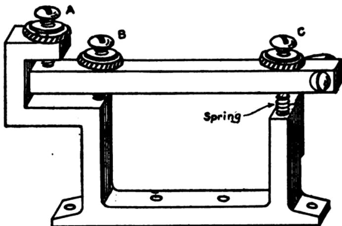
FIG. 87.—Sounder Frame with Lever in Position.
