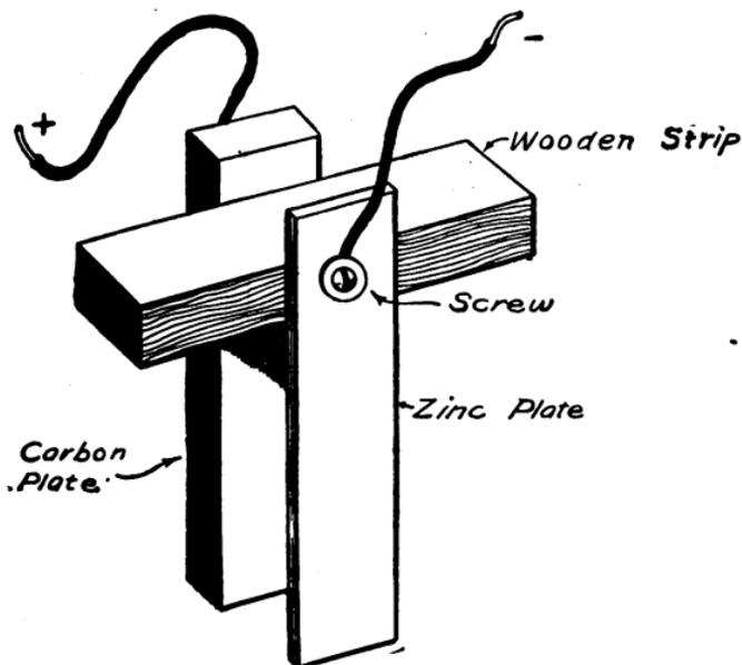
FIG. 28.—A Simple Home-made Cell.
