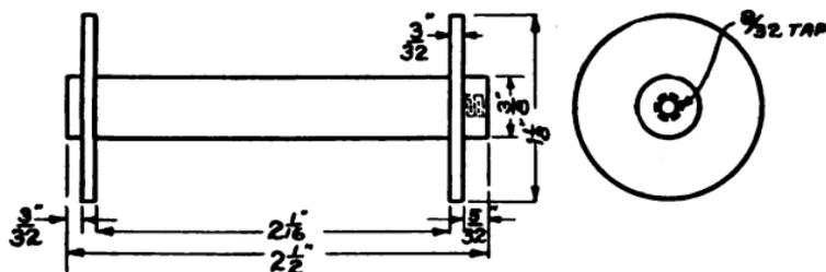
FIG. 145.—Details of the Electromagnet Bobbin.
