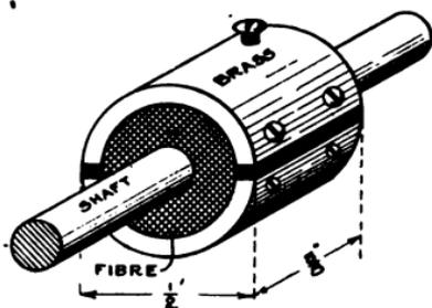
FIG. 126.—The Commutator.
