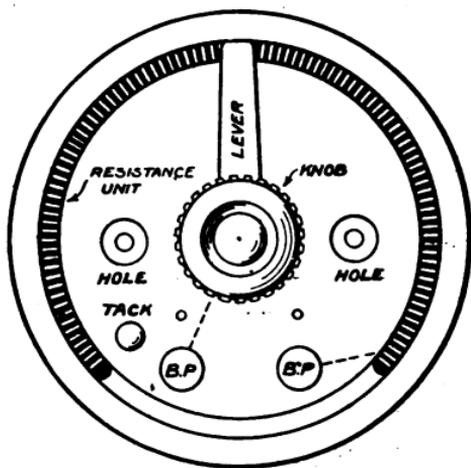
FIG. 77.—Top view of a small Battery Rheostat.
