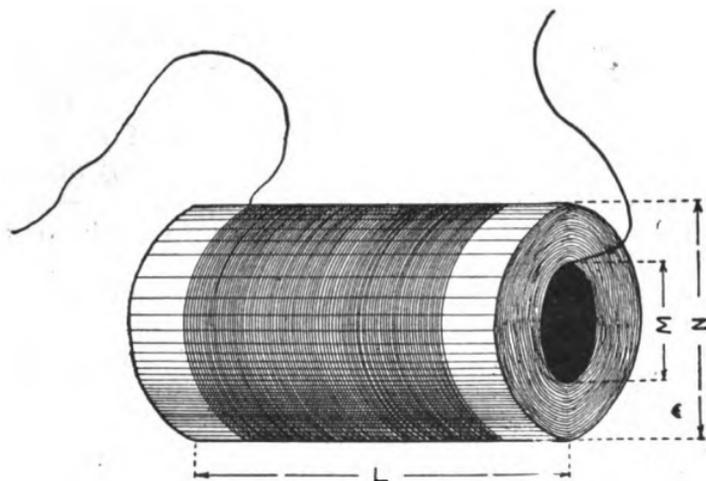
FIG. 111.—The Secondary Winding.
