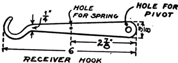
FIG. 95.—Details of the Receiver Hook.
