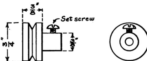
FIG. 130.—The Pulley.
