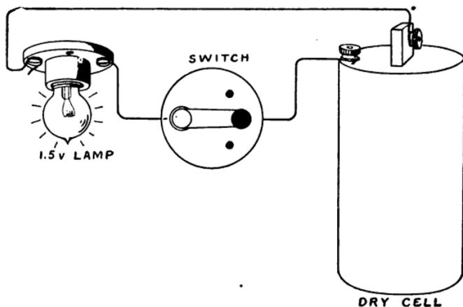
FIG. 153.—A Simple Lighting Arrangement.
