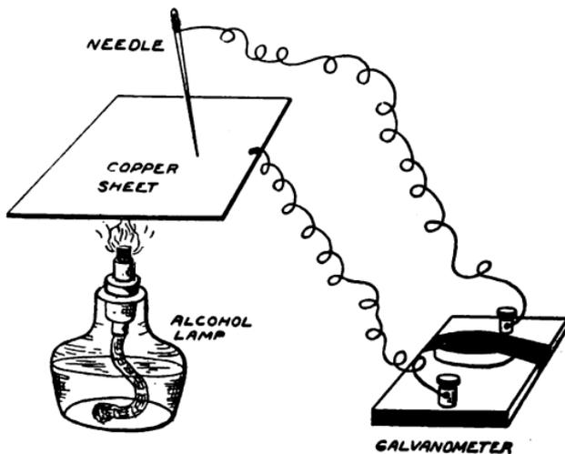
FIG. 187.—Generating Electric Current by Heat.
