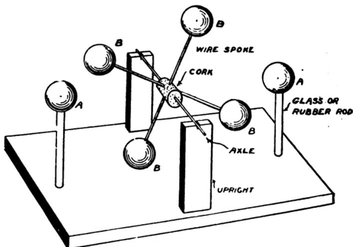
FIG. 194.—The Static Motor.
