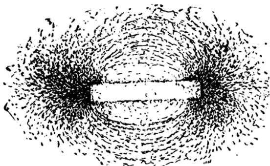
FIG. 180.—Magnetic Phantom showing the Lines of Force about a Bar Magnet.
