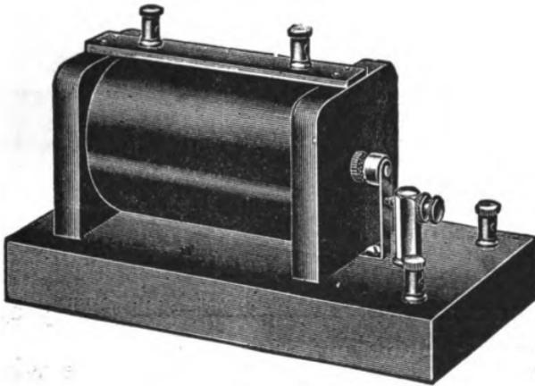
FIG. 109.—Induction or Spark Coil.
