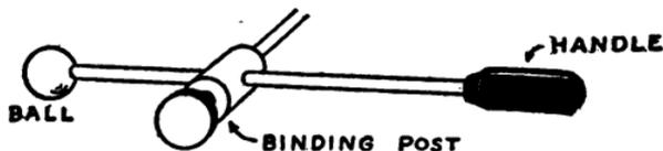
FIG. 11.—Showing how Binding Posts may be substituted for Round Balls on the Collector Rods.
