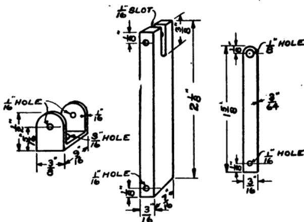
FIG. 149.—The Armature, Armature Bearing and Connecting Rod.
