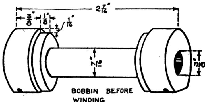
FIG. 98.—Bobbin for Medical Coil.
