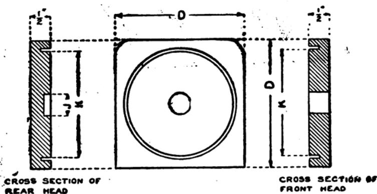
FIG. 113.—Details of the Wooden Coil Heads.
