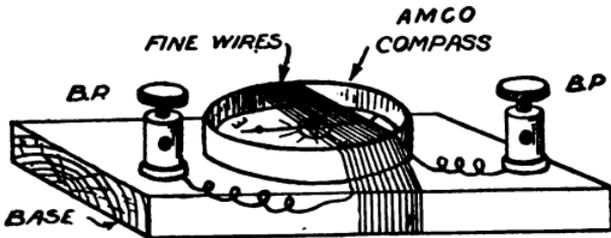
FIG. 67.—A Simple Galvanometer.
