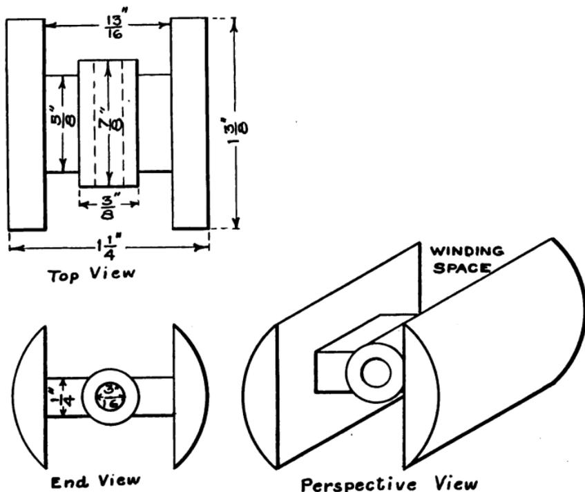
FIG. 125.—Details of the Armature.
