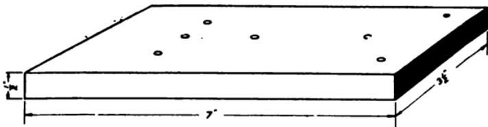
FIG. 144.—The Engine Base.
