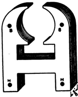
FIG. 135.—The Assembled Field ready for Winding.
