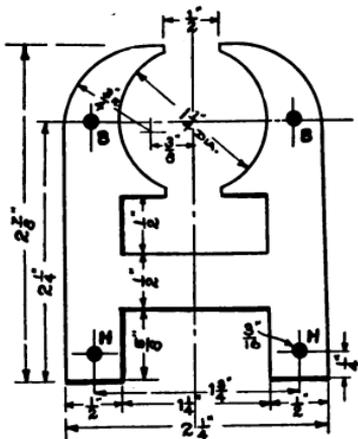
FIG. 134.—Details of the Field Frame.
