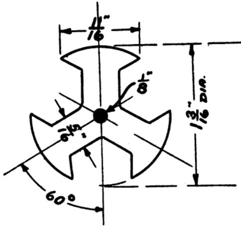
FIG. 136.—Details of the Armature Lamination.
