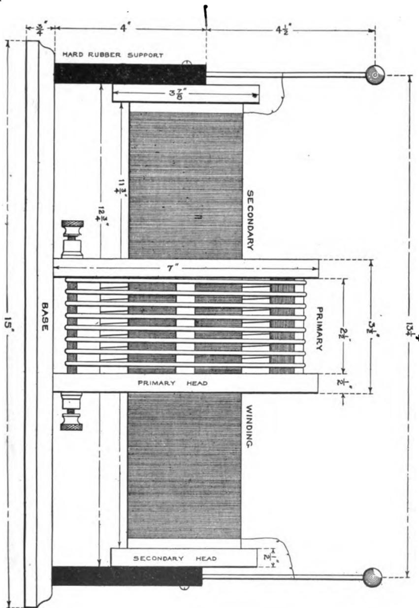
FIG. 175.—Front View of the completed Tesla Coil.
