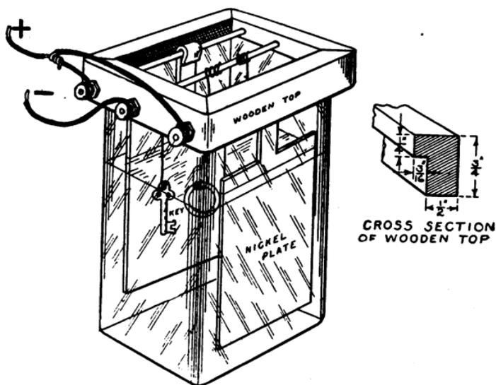
FIG. 186.—Electroplating Tank.
