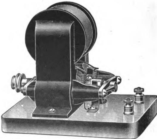
FIG. 132.—The Completed Dynamo.
