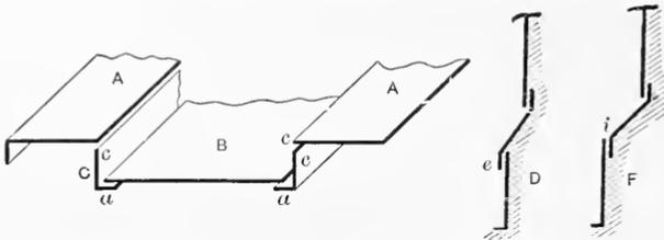
FIG. 173. Method of Stripping the Gothic Panel.
