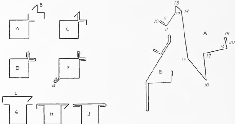
FIG. 411. Bending Corner and Middle Posts. FIG. 412. Forming Curb P in Fig. 409A.
