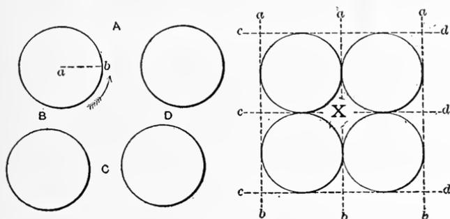
FIG. 4. Avoiding Waste in Material in Cutting Circles.
