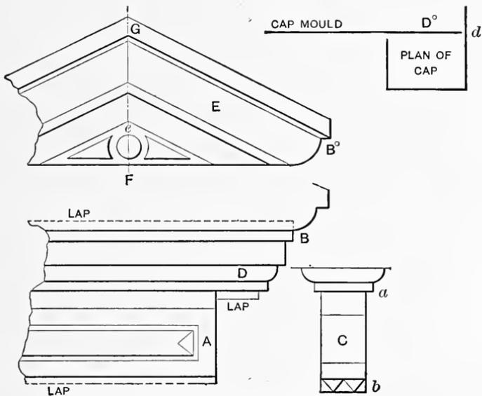
FIG. 122. Joining Various Parts of Window Cap.
