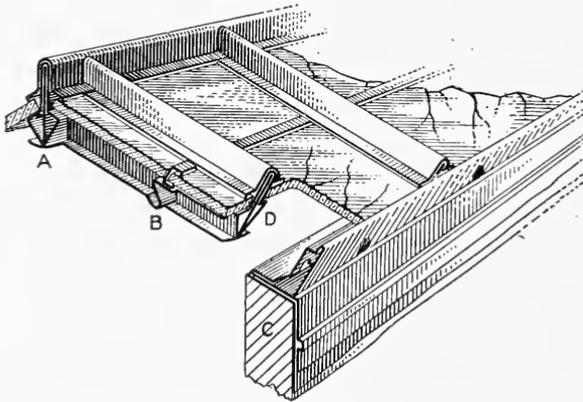
FIG. 308. Sectional View of Double Pitch Skylight.
