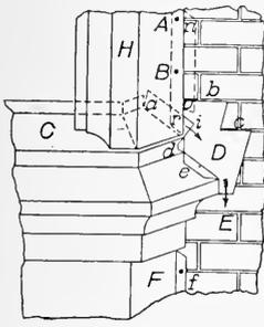
FIG. 505. Making Connections Water Tight.
