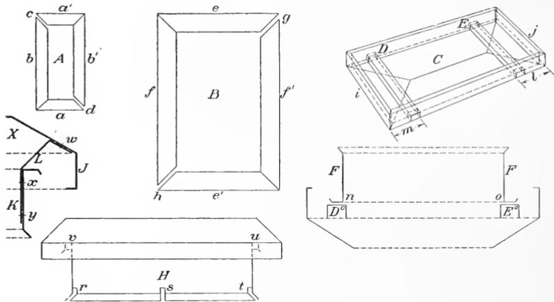
FIG. 391. Method of Assembling Ventilator and Curb.
