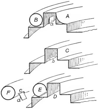
FIG. 568. Attaching a Curved Bead.
