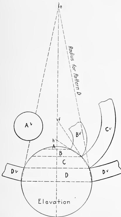
FIG. 517. Laying out Patterns for 10 inch Ball Scale 1½ inch to 1 Ft.
