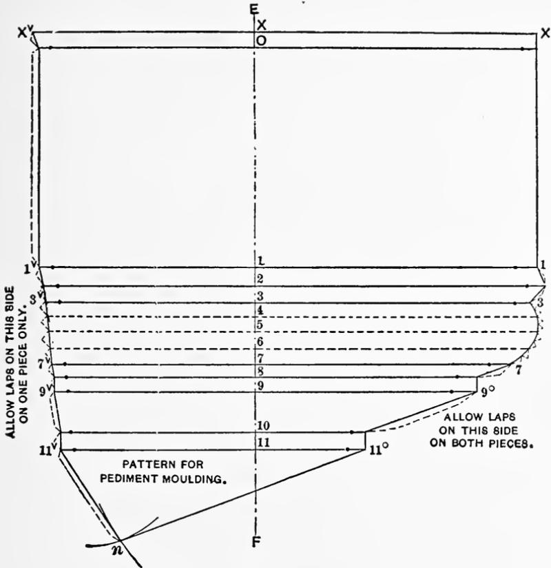
FIG. 118. Pattern for Raking Pediment Mold.
