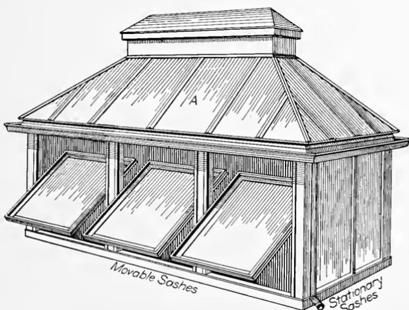
FIG. 456. Hip Ridge Ventilating Skylight with Movable Sash Turret.
