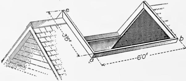
FIG. 296. Measurements for Frame for Ridge Skylight.
