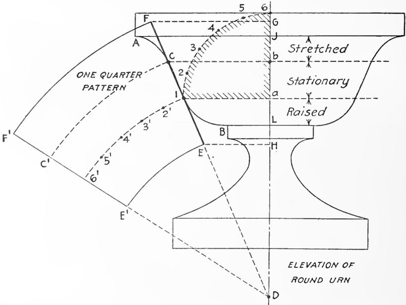
FIG. 558. Developing Pattern for Ogee in One Piece with Raised and Stretched Portion.
