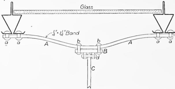
FIG. 314. Truss, Hinge and Raising Rod for Small Skylight.
