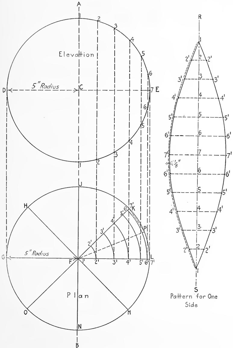
FIG. 534. Details and Gore Patterns for 10 Inch Ball.
