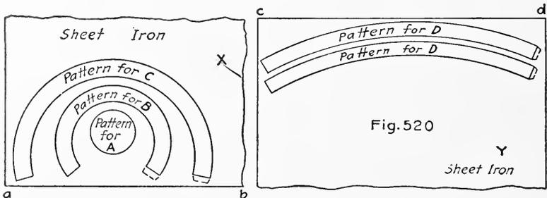
FIG. 520. Placing Patterns to Avoid Waste of Material.
