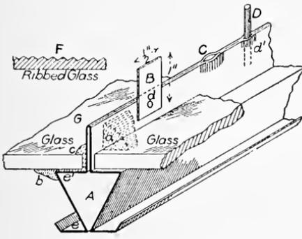
FIG. 290. Fastening Clip to Secure Cap Bar.
