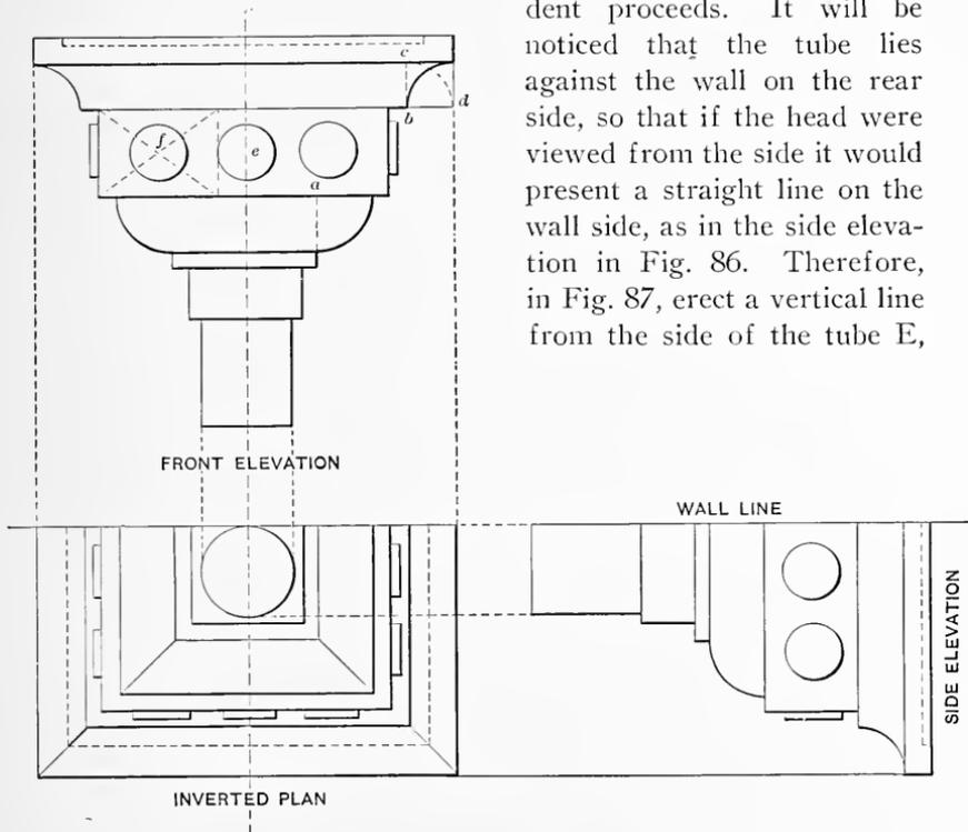
FIG. 86. Plan and Elevations of Square Leader Head
