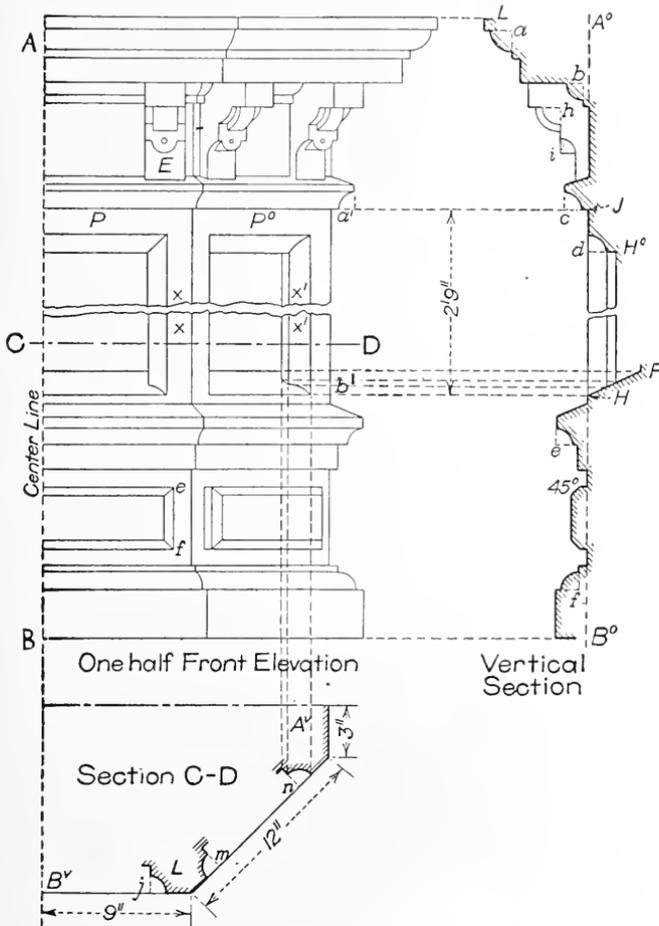
FIG. 465. Elevation and Section of Bay Window.
