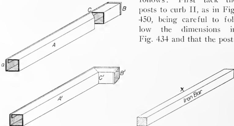
FIG. 449. Assembling and Soldering the Leaders.
