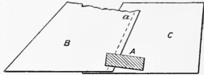
FIG. 21. Copper Improperly Placed to Sweat Seam.
