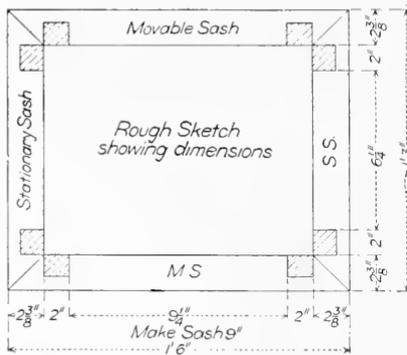
FIG. 434. Rough Sketch Showing Dimensions of Sash.
