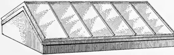
FIG. 294. Double Pitch Skylights for Flat Roofs.
