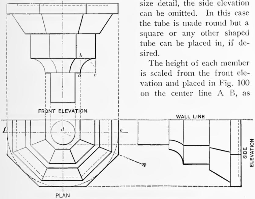
FIG. 99. Plans and Elevations of Octagon Leader Head.
