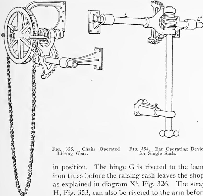
FIG. 355. Chain Operated Lifting Gear. FIG. 354. Bar Operating Device for Single Sash.
