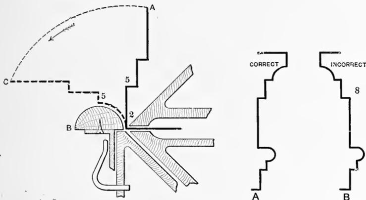
FIG. 68. Second Operation in Forming Cove. FIG. 69. Possible Error in Forming
