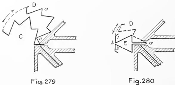
Bending Operation on Brake in Forming Common Bar for Skylight.
