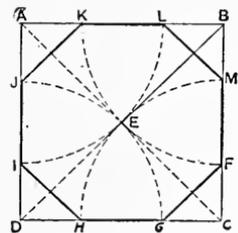
FIG. 57. Drawing an Octagon Within a Given Square.
