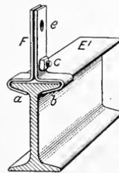
FIG. 136. Method of Fastening to Iron Beams.
