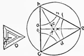
FIG. 34. Finding the Center of a Triangle.
