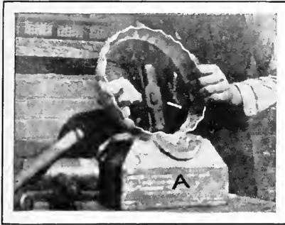
FIG. 526. First Operations in Raising Sections of Ball.
