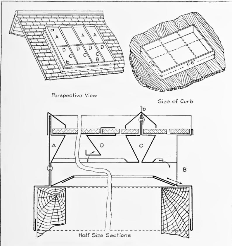
FIG. 251. Different Views and Detail of Flat Skylight.
