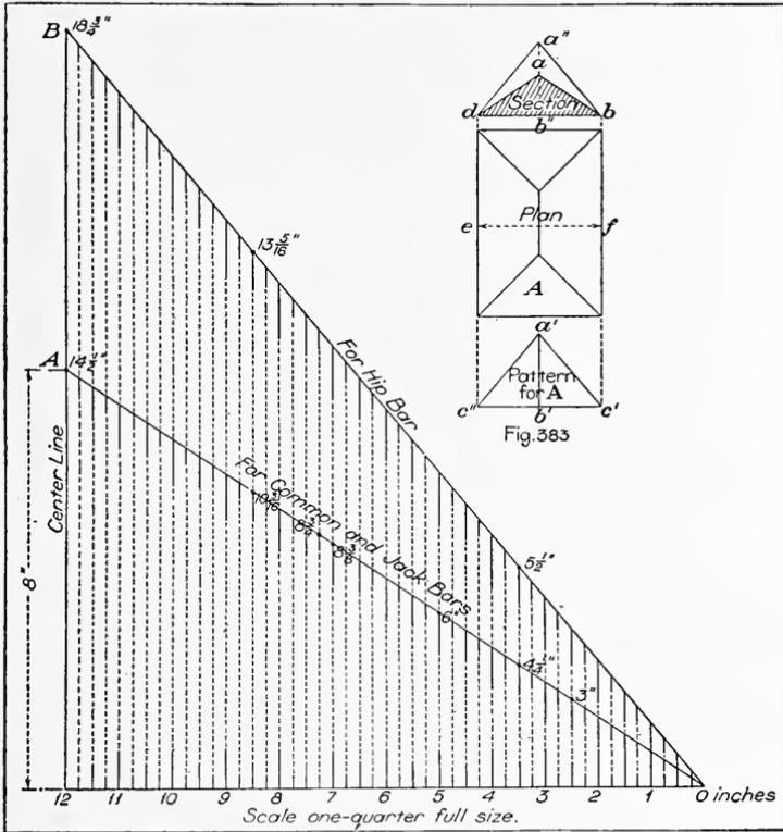
FIGS. 382-3. Method of Obtaining Lengths of Skylight Bars.
