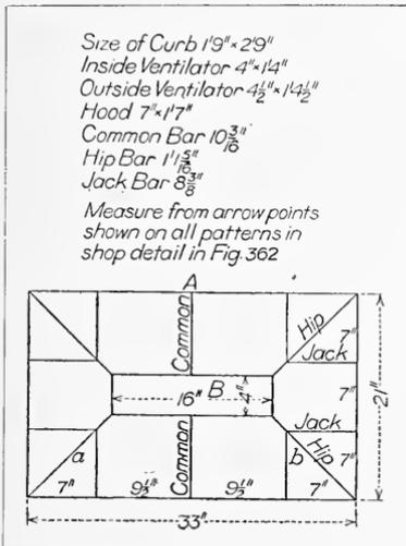
FIG. 377. Getting Various Dimensions of Skylight Parts.
