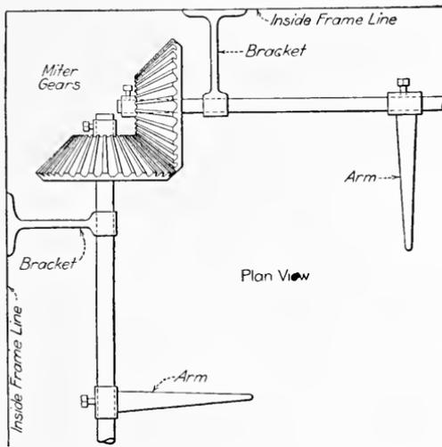
FIG. 357. Miter or Bevel Gear for Lifting Sash.
