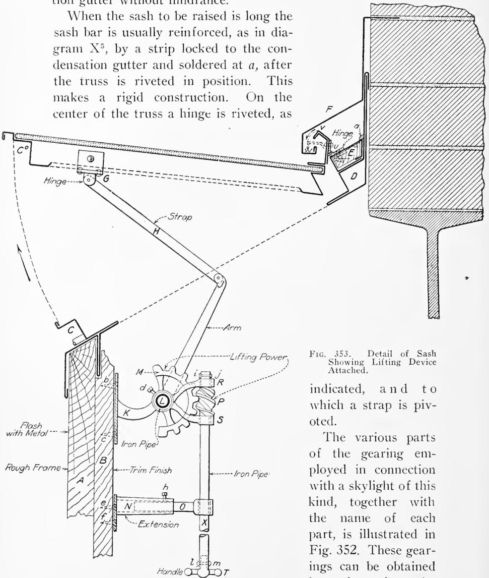
FIG. 353. Detail of Sash Showing Lifting Device Attached.
