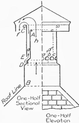
FIG. 250. Exhaust Ventilator.
