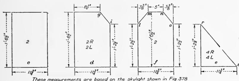
FIG. 398. Diagram Showing How to Compute Size of Glass Required for Skylight.
