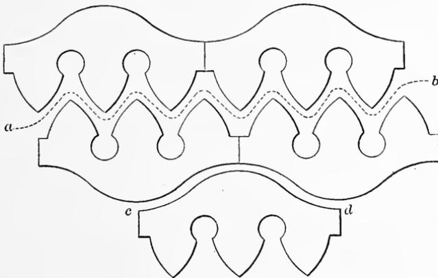
FIG. 12. Method of Cutting Fifth Templet.
