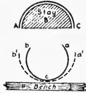
FIG. 536. Raising to Conform to Stay.
