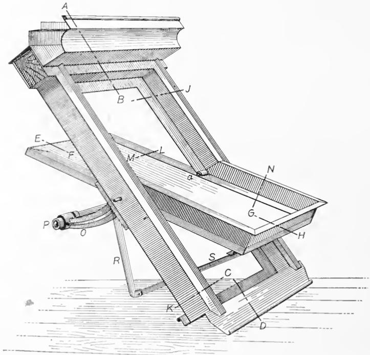
FIG. 461. Movable Sash Skylight Showing Gutter, Curb and Gearing in Position.
