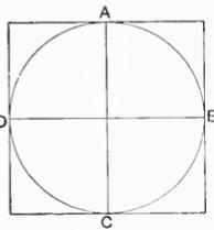
FIG. 53. Drawing a Square Outside of a Given Circle.
