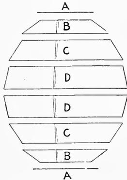
FIG. 523. Flares Rolled and Soldered Previous to Raising.
