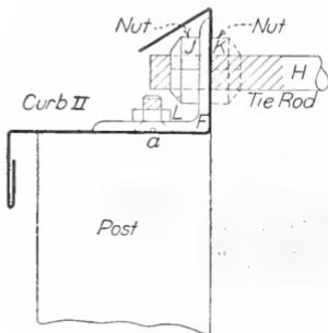
FIG. 457. Tie Rod in Upper Curb.
