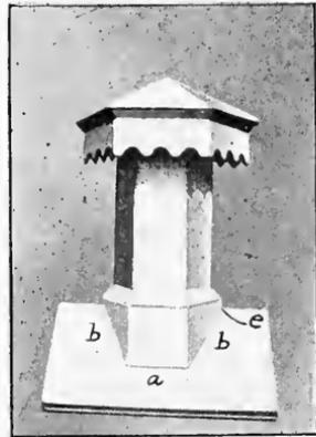
FIG. 239. Finished Hexagonal Ventilator.
