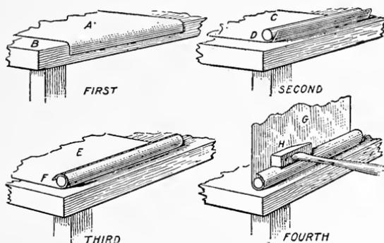
FIG. 77. Forming a Bead on a Bench.
