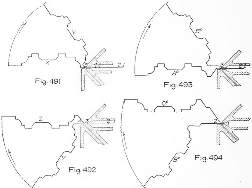
FIGS. 491 to 494 Inclusive. Final Operations in Forming Molding.
