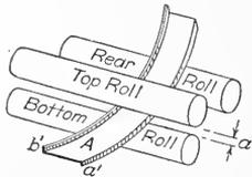
FIG. 562. Forming Edged Strips.
