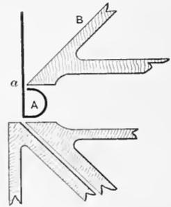
FIG. 76. Closing the Bead in the Brake
