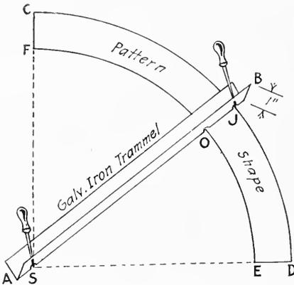
FIG. 519. Sheet Metal Trammels for Long Radii.
