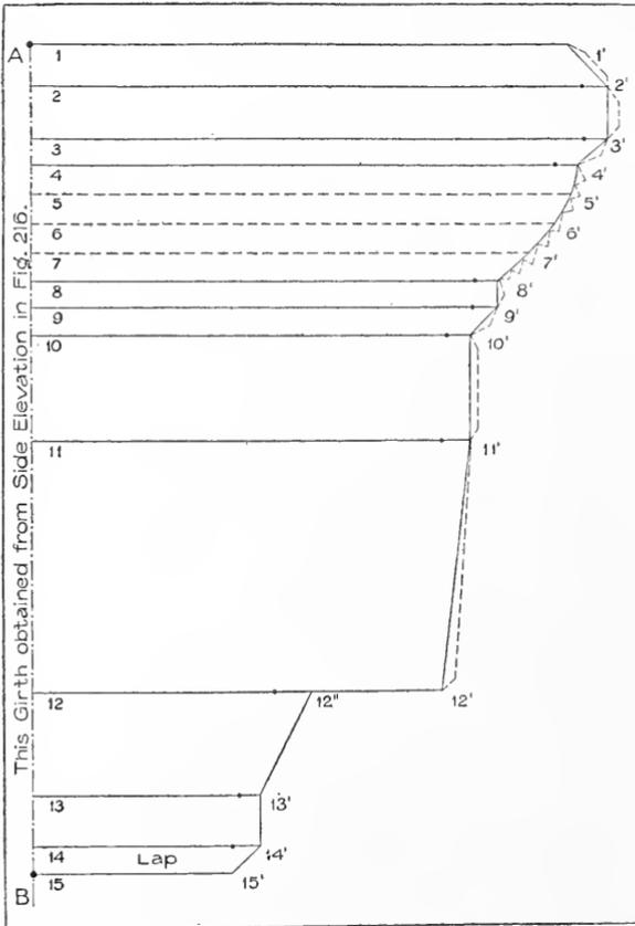
FIG. 219. Half Pattern for Crown Mold.
