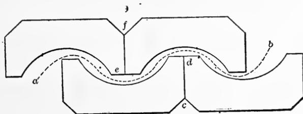
FIG. 6. Method of Cutting to Avoid Waste.
