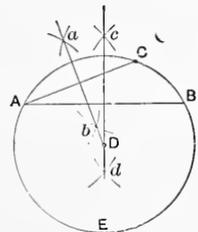
FIG. 48. Completing a Circle When Only Arc is Given
