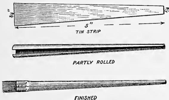
FIG. 16. Method of Making Acid Brush.
