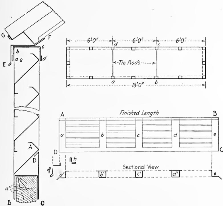
FIG. 418. Parts Constructed in Shop Ready to Send to Building. FIG. 419. Heavy Construction for Large Louvres. FIG. 420. Location of Tie Rods.
