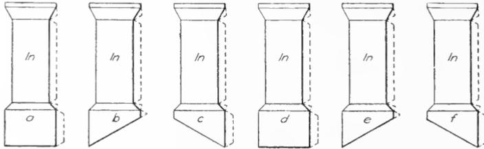
FIG. 240. Placing and Joining Laps on Ventilator Shaft Slides.
