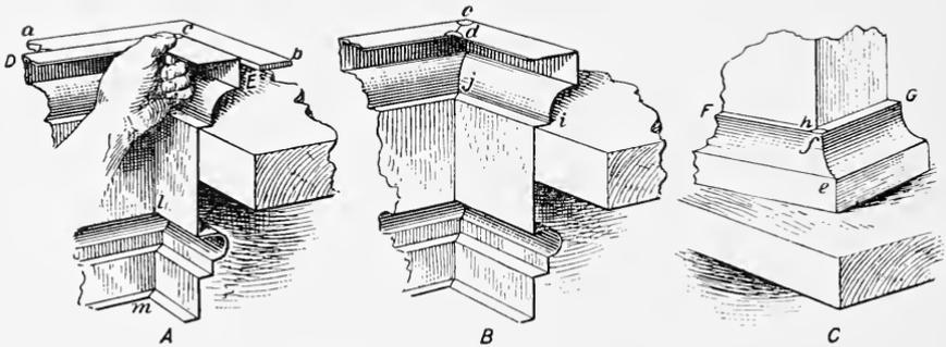
FIG. 71. Handling Miter on Bench in Making Joints.
