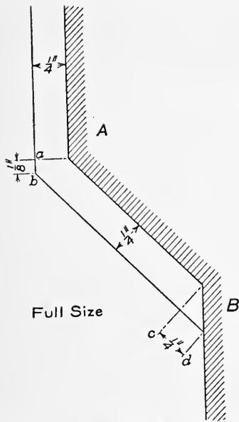
FIG. 514. Method of Making Allowance for Projection.
