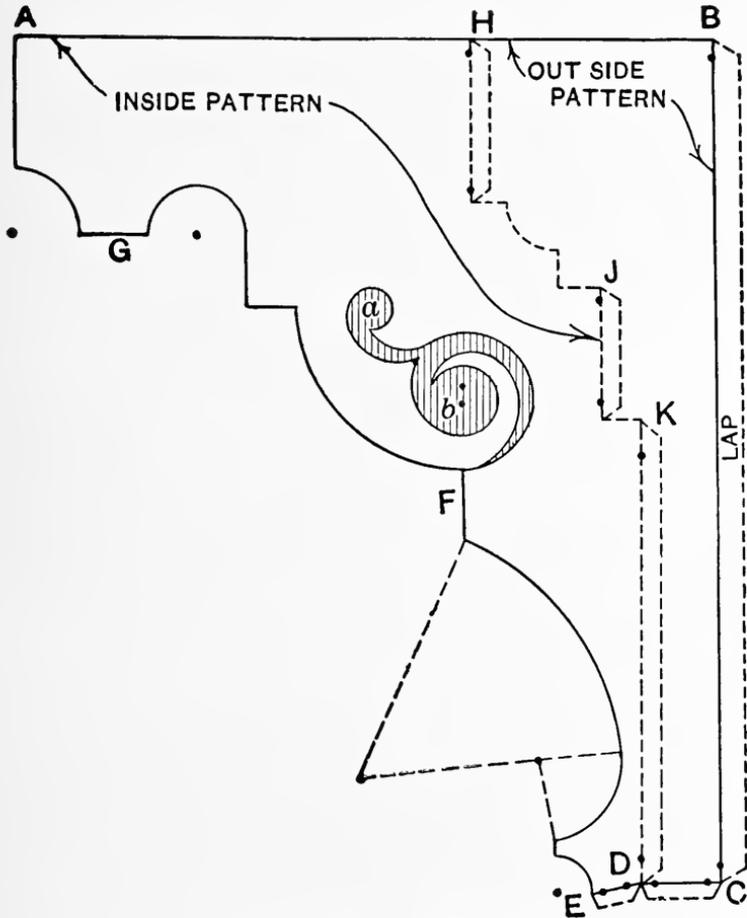
FIG. 142. Pattern for Bracket Sides.
