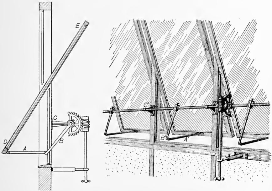
FIG. 460. Method of Attaching Gearing for Movable Skylights.
