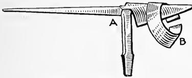
FIG. 521. Blow Horn Stake.
