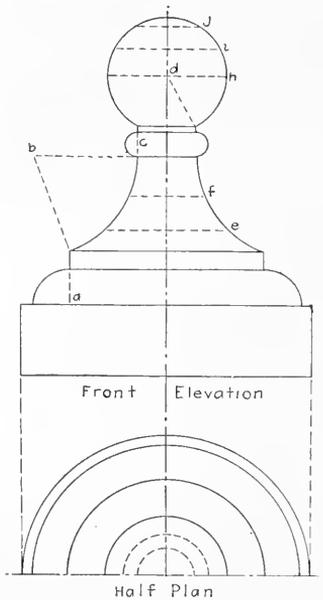
FIG. 543. Half Plan and Elevation of Round Finial—Scale  $1\frac{1}{2}$  Inches to Ft.
