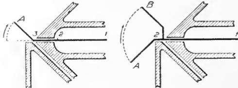
FIGS. 242-3. Operations in Bending Hood and Roof Piece Joining Miters.
