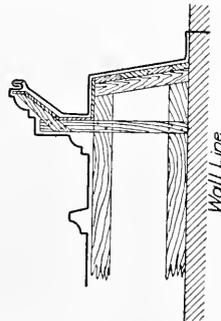
FIG. 509. Constructing Gutter.
