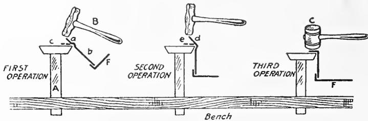
FIG. 554. Stretching the Circular Flange.
