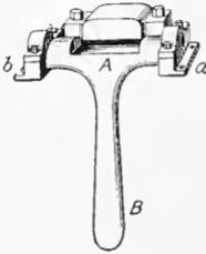
FIG 134. The Brace Bender.
