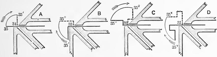
FIG. 131. Forming Drips on the Front Mold.
