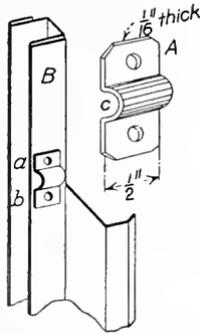
FIG. 464. Method of Fastening Hinge to Sash.
