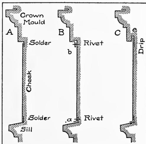
FIG. 228. Joining Cheek to Crown Mold.
