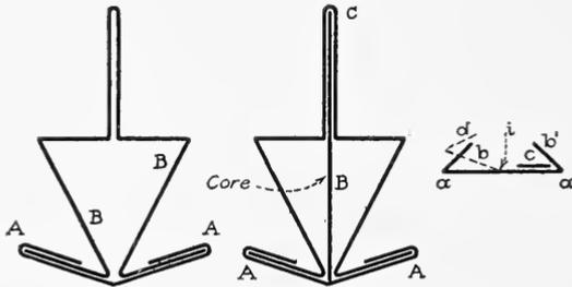
FIG. 298. Reinforced Bar. FIG. 299. Bar With Sheet Metal Core.
