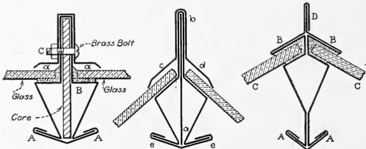
FIG. 300. Bar With Steel Core. FIG. 301. Ridge Bar With Sheet Metal Core. FIG. 302. Ridge Bar and Cap Combined.
