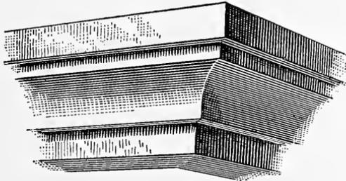
FIG. 85. Finished Molded Gutter Miter.
