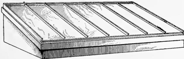
FIG. 297. Single Pitch Skylight for Flat Roof.
