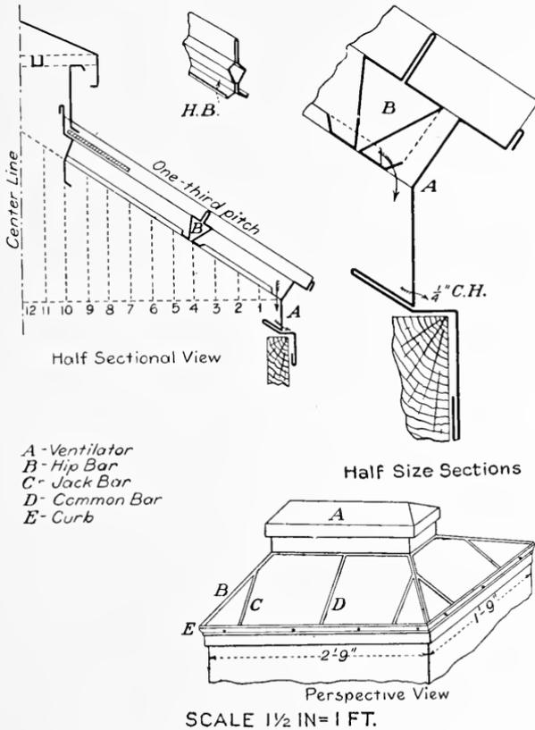
FIG. 358. Perspective and Sections of Hipped Skylight.
