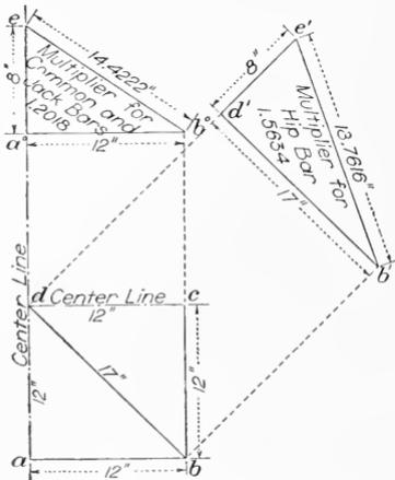
FIG. 386. Finding Length of Bars by Multipliers.
