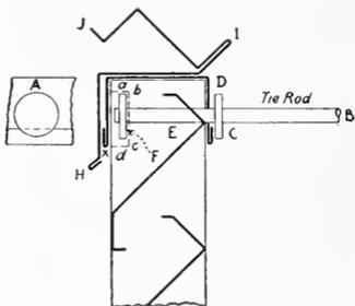
FIG. 421. Tie Rod Brace for Large Louvres.
