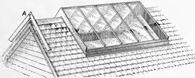
FIG. 295 Double Pitch or Ridge Skylight.
