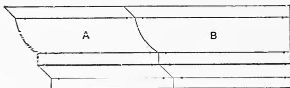
FIG. 119. Saving Time and Material In Cutting Caps.
