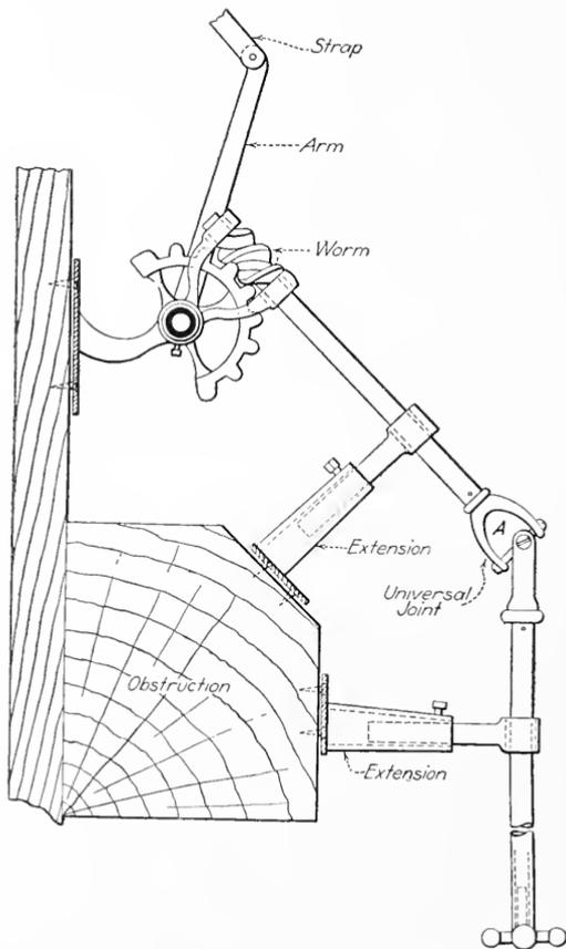
FIG. 356. Application of Universal Joint to Lifting Gear.
