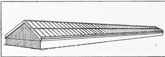
FIG. 309. Double Pitched Skylight With Cross Clips.
