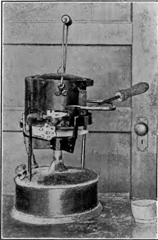
FIG. 11. Gasoline Fire Pot for Heating Soldering Irons.
