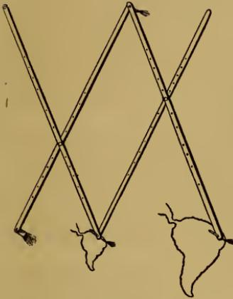
For enlarging and reducing all kinds of diagrams and engravings, no appliance is as simple and as accurate as the pantograph, illustrated by the accompanying cut, which represents this instrument in use for enlarging a map of South America.
