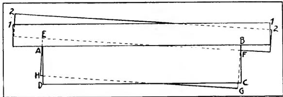
Fig. 206. Method of Using the Winding-Sticks.
