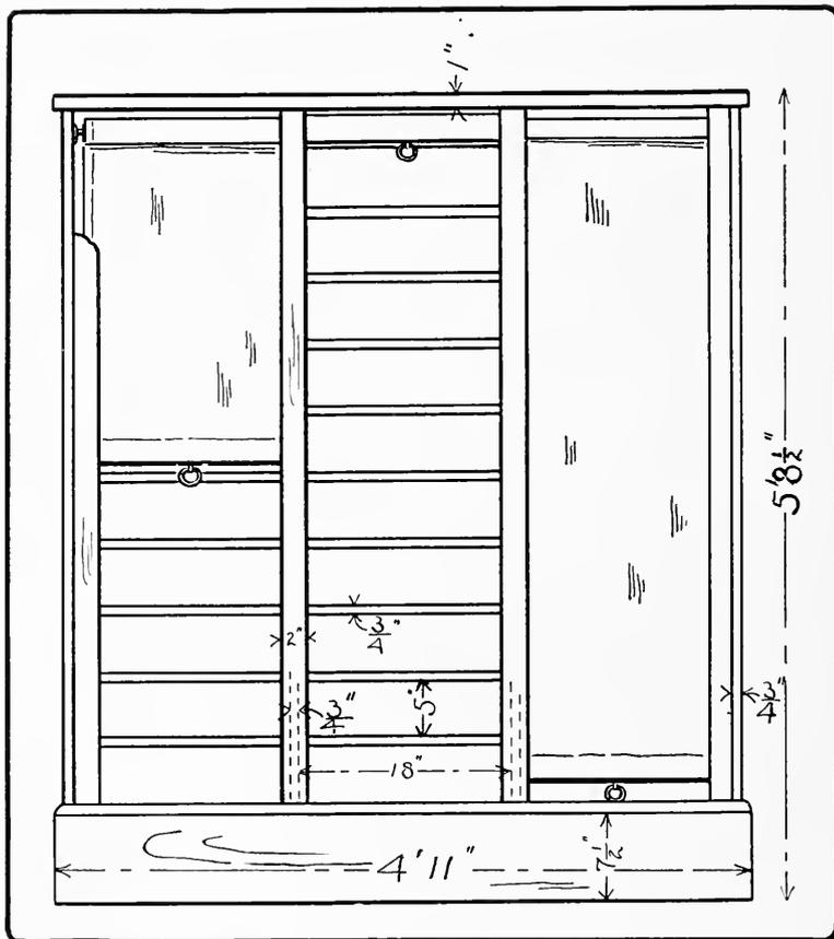
Fig. 241. An Inexpensive Locker for Unfinished Work.
