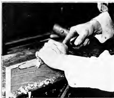
Fig. 275. Stop Chamfering.
