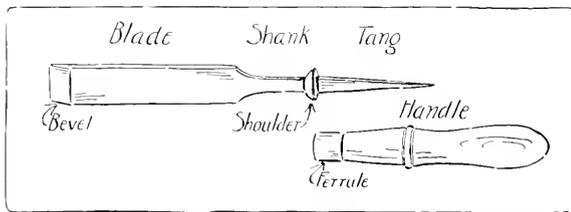
Fig. 65. Firmer-Chisel.
