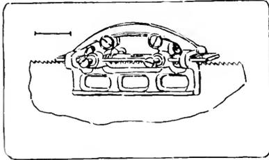
Fig. 97. A Saw-Jointer.
