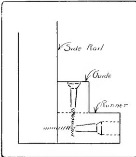
Fig. 295. Drawer Mechanism.
