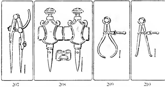
Fig. 207. Winged Dividers. Fig. 208. Beam-Compass or Trammel Points.
