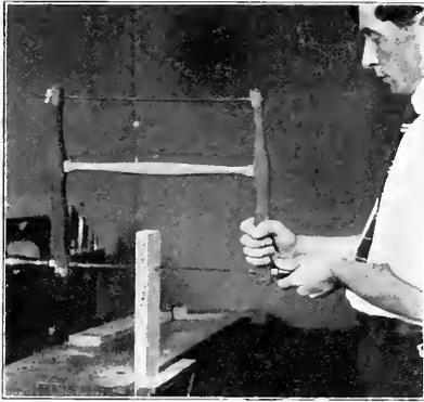
Fig. 95. Using a Turning-Saw.
