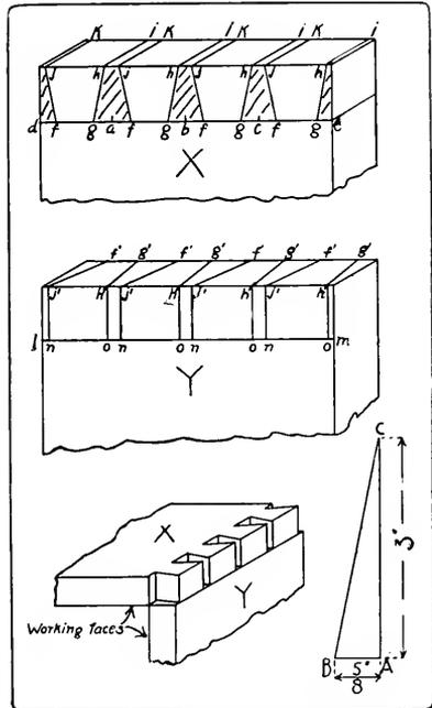
Fig. 250 Laying Out a Dovetail Joint.
