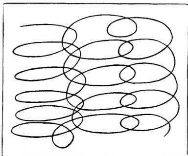
Fig. 304. Direction of the Pad in French Polishing.
