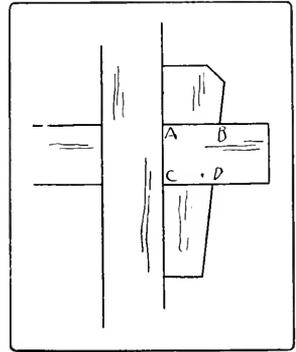
Fig. 252. Keyed Mortise-and-Tenon Joint.
