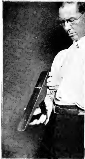
Fig. 102 Sighting Along the Sole of Jack-Plane
