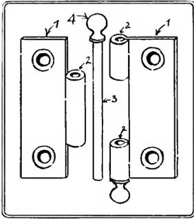
Fig. 234. Parts of a butt-hinge.
