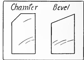
Fig. 271. Difference Between Chamfer and Bevel.
