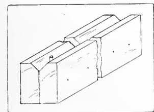
Fig. 274. Trough for Planing Chamfers.
