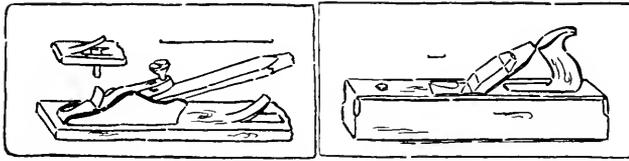
Fig. 99. Adjustable Chisel-Gage. Fig. 100. Wooden Bench-Plane.
