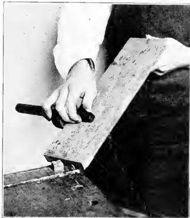
Fig. 214. Using the Marking-Gage.
