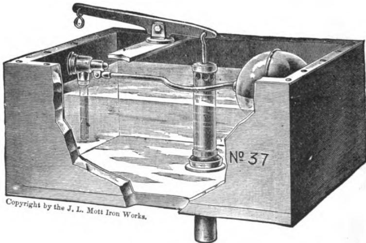
FIG. 24.—FLUSHING CISTERN.
