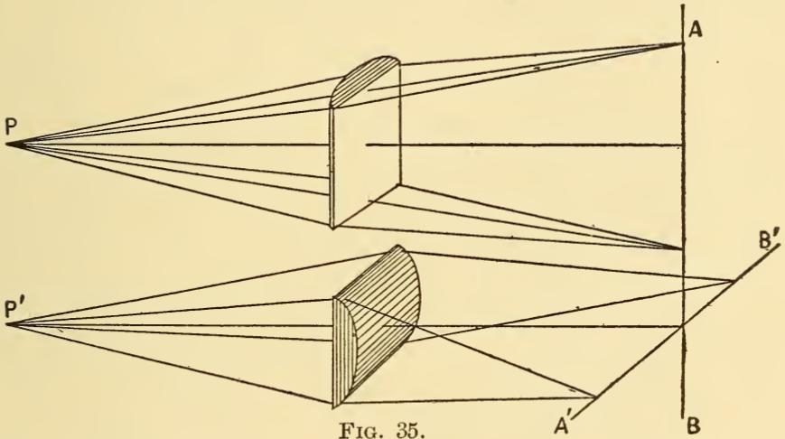
power, and if we combine them so that the rays after deviation by the first lens pass immediately through the second lens, the effect of both lenses will be to cause the rays to meet in the *point* where the lines intersect; for the rays must all pass through both lines. In other words, two equal cylindrical lenses placed with their axes at right angles are equivalent
