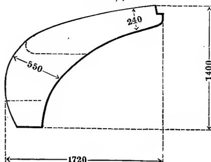
During a thirty days' siege it was calculated that the armour of the turret would be struck by from 1,000 to 1,500 shells, and it was considered entirely sufficient if a quadrant of the turret under trial withstood 200 long shells from the 5.9 in. hooped gun at a distance of 1,093 yards.
