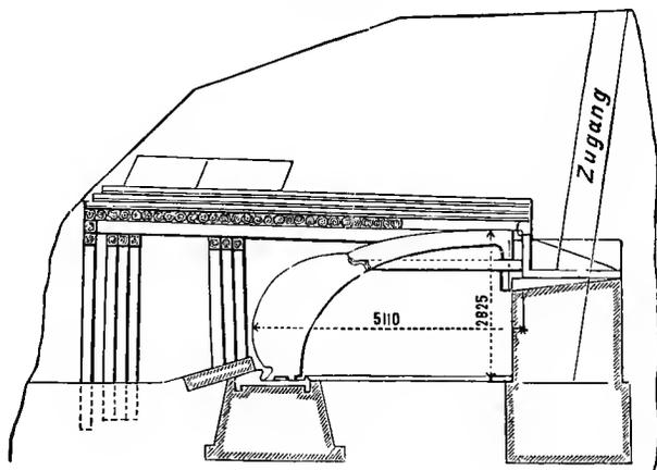
Target: The trial plate formed part of the cupola of the turret previously described as ordered by the Dutch Government. It was placed between four other side-plates and a roof-plate, so as to form half a turret, which rested at the rear against three strong pillars of masonry, connected with the armour by three stout specially cast struts.
