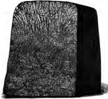
It will be noticed in this figure, which shows the section of a chilled bar, that the exterior layer is of a fine fibrous character, which passes without visible lines of separation into the granular structure of the so-called mottled iron, which in turn gradually assumes the character and fine crystalline structure of the soft grey iron.
