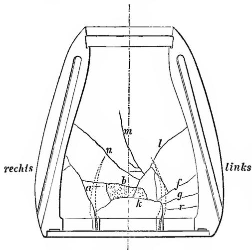
**Summary:** The first part of the trial had showed once more that steel shot of small calibre break up on striking an oblique surface of armour, in the same way as the 16.9 in. shell fired in April.
