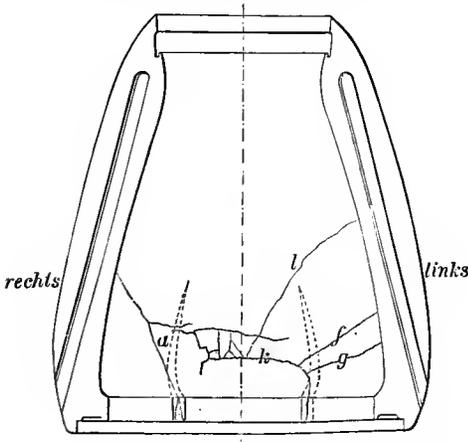
Back of the plate: A new crack running upwards and to the left from the centre line was seen apparently in connection with the hair crack *l* on the front surface; *k* was lengthened to the lower edge of the plate, and between *k* and *b* a nest of several small cracks had appeared owing to which a small wedge-shaped piece weighing about 4.4 lb., shown in dotted lines, had fallen from the inner surface. It measured 3.5 by 4.3 by 3.2 in.
