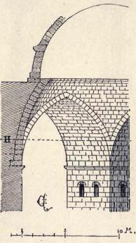
3. SECTION OF A PENDENTIVE ON THE DIAGONAL A TO B IN PLAN, FIG. 1
