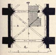
7. PLAN OF VAULT ON INTERSECTING ARCHES
