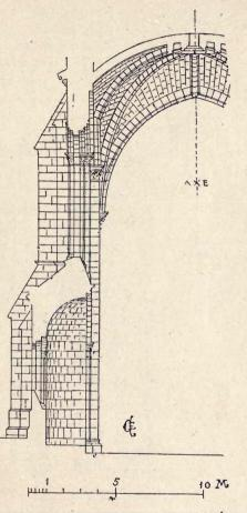
21. TRANSVERSE SECTION OF A BAY OF LA STE. TRINITÉ AT ANGERS which ensured the solidity of the ancient buildings,
