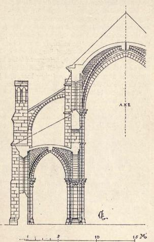
23. SECTION OF A THREE-AISLED CHURCH VAULTED ON INTERSECTING ARCHES WITH FLYING BUTTRESSES
