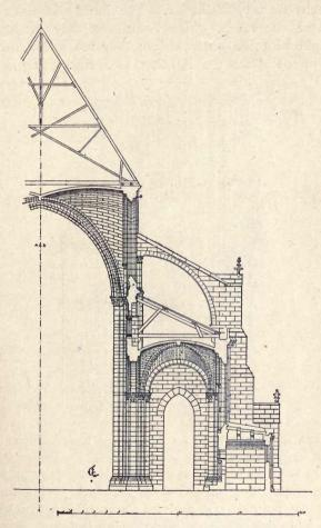
41. SENS CATHEDRAL. SECTION OF A BAY OF THE NAVE that of Sens. The structure is one of five aisles,
