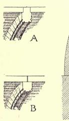
sustain the vault by 7 distributing its thrusts over four points of support.
